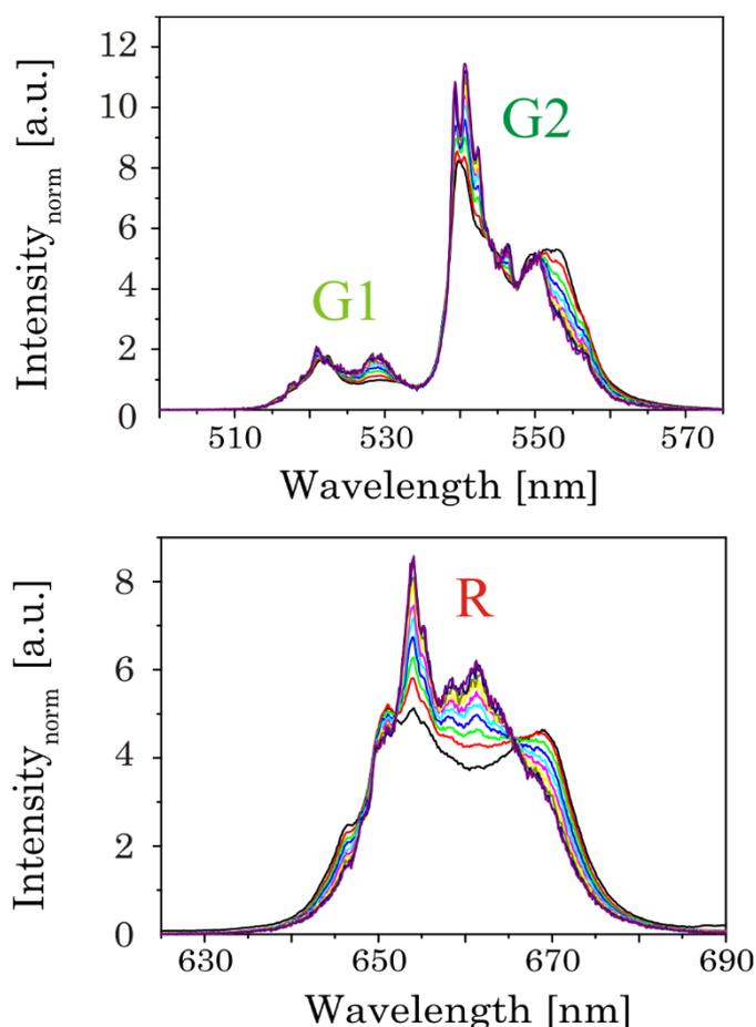
Fig. 12: TRANES of annealed UCNP<sub>300</sub> for (up) G1 and G2 luminescence as well as (below) of R luminescence are shown ( $\lambda_{\text{ex}} = 976$  nm). The delay after the laser pulse was varied between 0  $\mu\text{s}$  and 2000  $\mu\text{s}$  (displayed by the colors in 120  $\mu\text{s}$  steps).
