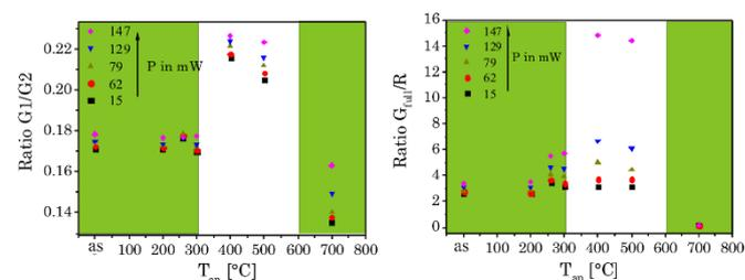
Fig.8: Peak ratio G1/G2 (left) and  $G_{\text{Red}}/R$  (right) versus annealing temperature at different laser power  $P$ . The green inset represents the alpha phase and the white inset the beta phase of the host lattice ( $\lambda_{\text{ex}} = 976 \text{ nm}$ ).
