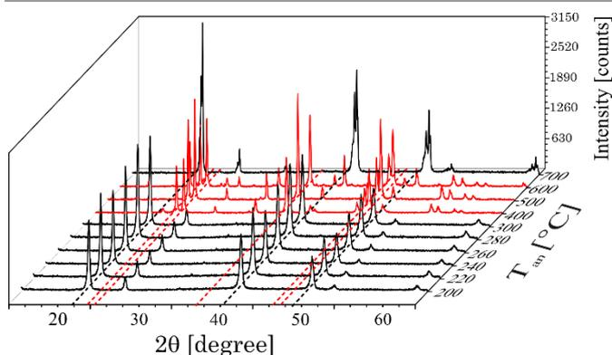
Fig.3: Suited selection of X-ray diffraction patterns of UCNP<sub>x</sub> after annealing between 200°C <  $T_{\text{an}}$  < 700°C for 5h. The black dotted lines correspond to the position of reflexes of the cubic phase whereas red dotted lines correspond to the position of reflexes of the hexagonal phase, respectively.
