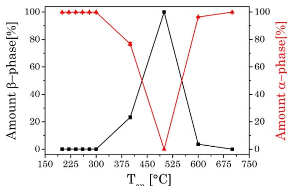
Fig.4: Amount of  $\alpha$ - and  $\beta$ -phase in correlation to temperature of the thermal treatment, calculated on the intensity of the different XRD reflexes of  $\alpha$ - and  $\beta$ -phase.
