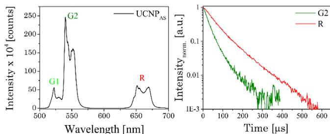
Fig.2: (left) Upconversion luminescence spectrum of the as-synthesized UCNP<sub>AS</sub>. The spectrum was recorded from a powdered sample with  $\lambda_{\text{ex}} = 976$  nm (power density of 191 mW/cm<sup>2</sup>). (right) Normalized upconversion luminescence decay kinetics of the Er<sup>3+</sup> emission bands G2 and R of UCNP<sub>AS</sub>.
