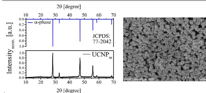
Fig.1: (left) The XRD diffractogram of as-synthesized UCNP<sub>AS</sub> (and the corresponding reference data from JCPDS) indicate that the sample is composed of the pure cubic  $\alpha$ -phase. (right) SEM image (500nm scale) of UCNP<sub>AS</sub>.
