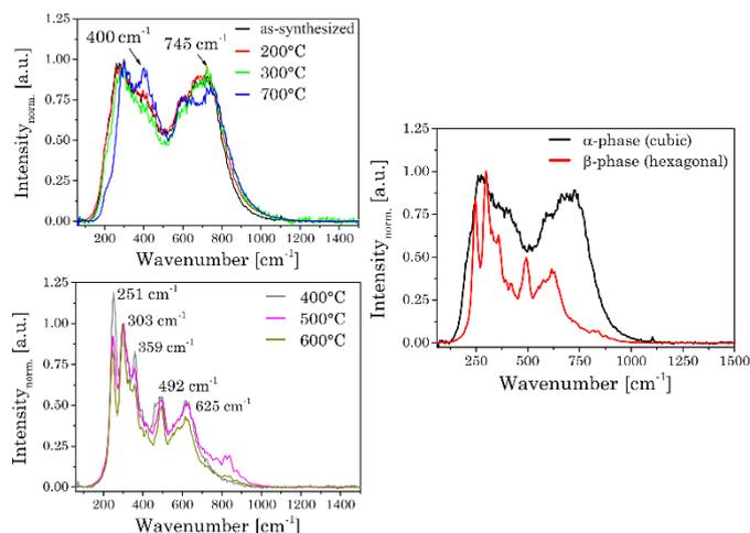
Fig.5: (left) Normalized Raman spectra of as-synthesized  $\text{UCNP}_{\text{AS}}$  and annealed  $\text{UCNP}_x$ . (right) Representative Raman spectra of  $\alpha$ - and  $\beta$ -phase.
