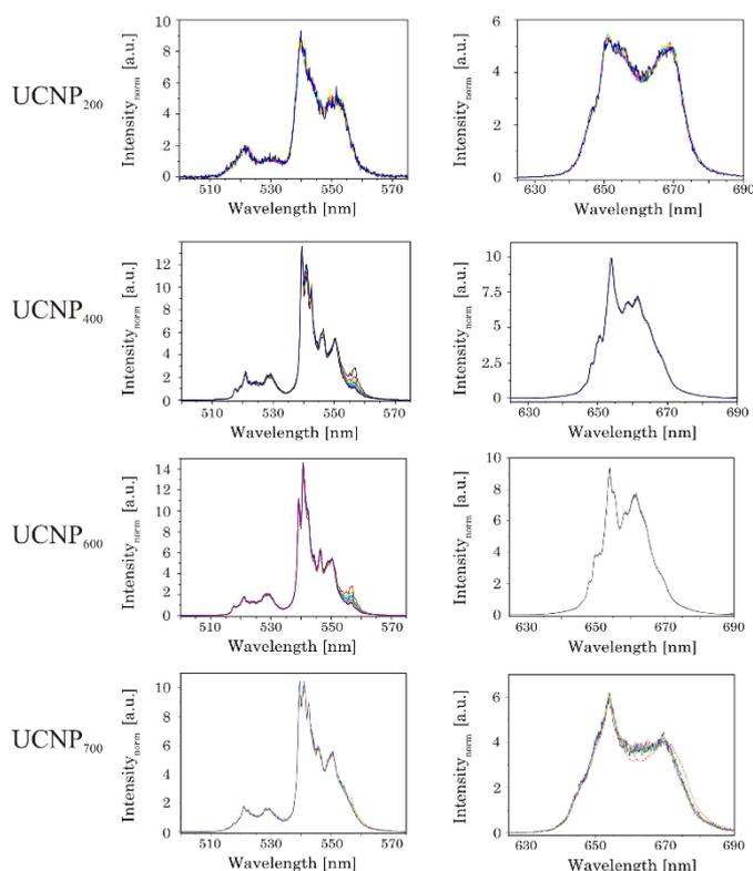
Fig. 11: TRANES of annealed UCNP<sub>x</sub> (200°C < x < 700°C) for (left) G1 and G2 luminescence as well as (right) of R luminescence are shown ( $\lambda_{\text{ex}} = 976$  nm). The delay after the laser pulse was varied between 0  $\mu\text{s}$  and 2000  $\mu\text{s}$ .
