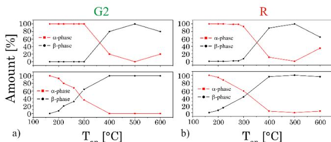
Fig. 13: Variation of the amount of different crystal phase ( $\alpha$ - and  $\beta$ -phase) calculated out of the TRANES analysis at delay times after the laser pulse (top: 0  $\mu$ s and bottom: 500  $\mu$ s) for emission band G2 (a) and R (b).
