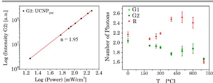
Fig. 7: (left) Dependence of upconversion luminescence intensity on laser power for G2 related emission of UCNP<sub>200</sub>. (right)  $n$ -values determined for the emission bands G1, G2, and R for UCNP<sub>x</sub> annealed at different  $T_{\text{an}}$ .
