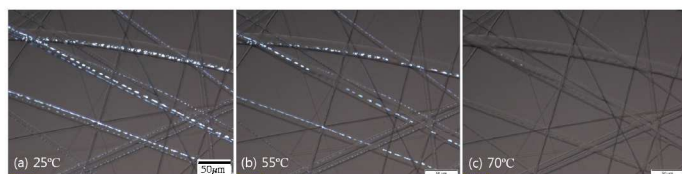
Fig. 7 Transmission polarizing microscopy images (polarizers are slightly decrossed to better visualize the fibers) of surfactant-free dual-core fibers with 5CB and E7 next to each other, heated until first the 5CB core, then the E7 core has turned isotropic.
