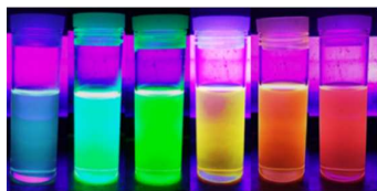
Fig. 2 Photographs of highly luminescent CdSe NCs of various sizes synthesized from cadmium deoxycholate precursor through the continuous mode in supercritical hexane (at P = 10 MPa; 250^\circ\text{C} < T < 310^\circ\text{C} ) showing emissions from blue to red regions of the visible spectrum (using UV-lamp at an excitation wavelength of 365 nm).
