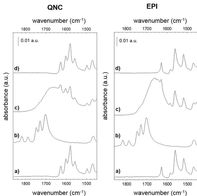
Fig. 9 Reflection FTIR spectra of QNC and EPI films before and after B7 incubation. a) Pristine hydrogen-bonded pigment film, b) Pristine B7, c) Pigment films incubated with B7, d) After incubation with B7, following washing.
