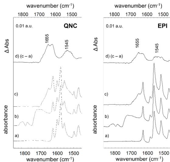
Fig. 4 RC bioconjugation to H-bonded semiconductors traced by FTIR spectra of RC-quinacridone (left) and RC-epindolidione hybrid systems (right): a) the pristine organic semiconductors; b) SUB linked to semiconductors; c) RC bioconjugated to semiconductor surfaces by SUB linker. d) Difference spectrum between (c) and (a).
