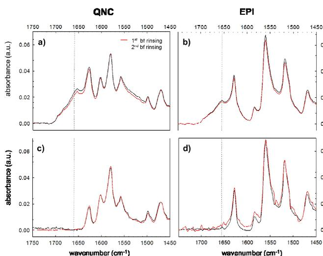
Fig 5 IR spectra after subsequent washing steps of bioconjugated a) and c) and physisorbed b) and d) RC samples both with quinacridone and epindolidione substrates. Washing was performed with PBS, pH 7.2.
