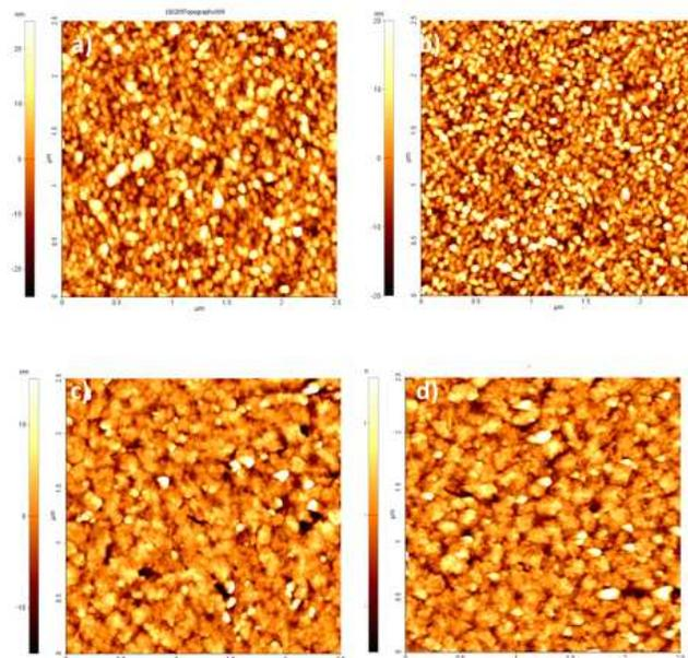
Fig. 10 AFM images of a) QNC functionalized with B7; b) QNC with B7 and streptavidin; c) EPI with B7; d) B7 and streptavidin
