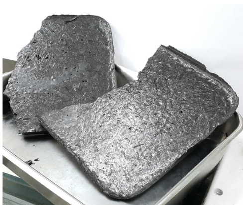
Figure SI 1. Solidified graphene mixture with NMMO m at room temperature after one month later.
