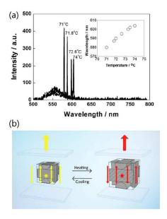
**Fig. 5** (a) Typical laser emission spectra for elevated temperatures in Cell-2. Peak lasing wavelengths collected at different temperatures (inset). (b) Schematic illustration of BPII laser tuning under thermal stimuli.
