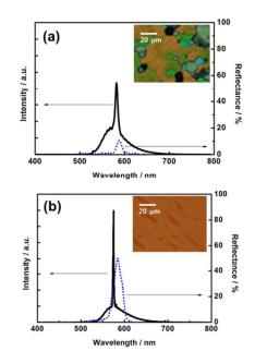
Fig. 4 Typical reflectance due to the lattice plane (100) and emission spectra for (a) Cell-1 and (b) Cell-2. Typical POM images (inset).
