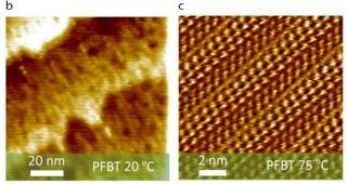
Fig. 1 a) Structures of the two SAM molecules used in this study. b) STM image of partially ordered PFBT SAMs on Au(111) formed at room temperature (constant current mode, 5 pA setpoint, 200 mV bias). c) STM of PFBT SAMs on Au(111) formed at 75 °C showing long range order 5 (constant current mode, 6.5 pA setpoint, 20 mV bias).
