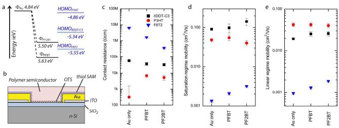
Fig. 4 a Energy levels of the (modified) electrodes and the polymer semiconductors. b Schematic of the OFET structure. c Contact resistance, d saturation regime mobility and e linear regime mobility of the devices made with gold or SAM-modified electrodes and the three semiconducting polymers IIDDT-C3 (black squares), P3HT (red circles) and F8T2 (blue triangles).
