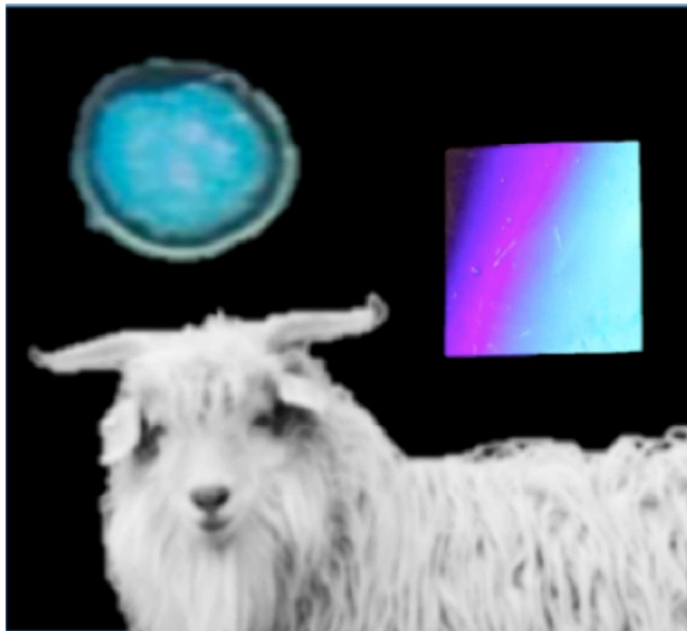
Cashmere-derived keratin is extracted in water solution and then processed with slow drying technique to obtain flexible, transparent, conformable optical elements. 136x124mm (300 x 300 DPI)
