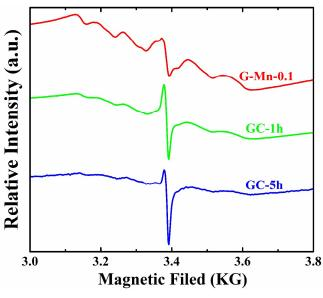
**Fig. 2.** Electron paramagnetic resonance (EPR) spectra of glass sample G-Mn-0.1 and glass-ceramic samples GC-1h and GC-5h measured at 85 K.
