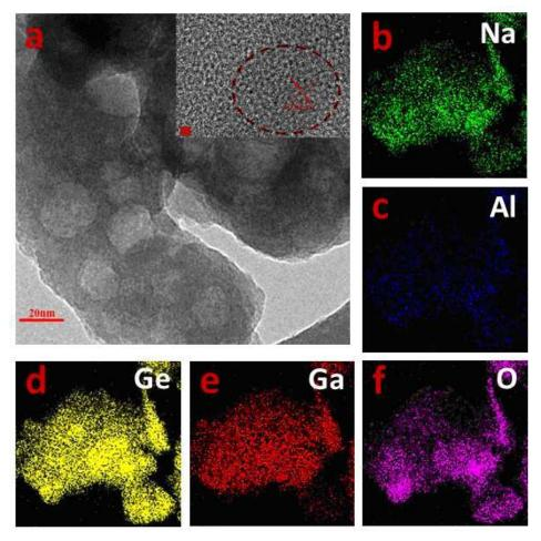
**Fig. 11.** (a) High resolution TEM image of glass ceramic sample GC-5h, scale bar is 20 nm; Inset: the HR-TEM image of the sample, scale bar 2nm. Red circle denotes the boundary between glass and crystal phases. The distance between neighbored crystal lattice fridges is ∼0.328nm, and it corresponds to the (002) crystal facet of albite Na(Al,Ga)Ge₃O<sub>8</sub> solid solution compound. (b)-(f) Two-dimensional elemental mapping of the distribution of Na, Al, Ge, Ga, and O, respectively.
