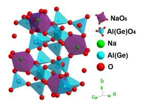
Fig. 1. Unit cell of NaAlGe<sub>3</sub>O<sub>8</sub> drawn on basis of crystallographic data on ICSD# 61170.
