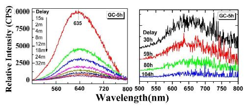
**Fig. 9.** Afterglow spectra of the glass sample GC-5h. The samples were pre-irradiated with an UV-254nm lamp for 5 min and measured at different delay times (15 seconds to 104hours) after removing the lamp.
