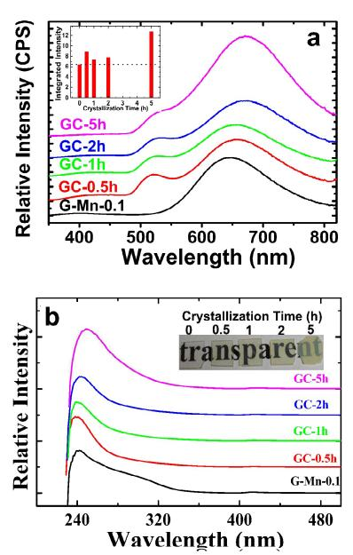
Fig. 7. (a) PL spectra ( $\lambda_{ex} = 250$  nm) and (b) Excitation spectra ( $\lambda_{em} = 650$  nm) of glass sample G-Mn-0.1 and glass-ceramic samples GC-0.5h, GC-1h, GC-2h and GC-5h. The curves were moved vertically for clarity. The inset of Fig. 7a shows the dependence of integrated PL intensity on crystallization time while the inset of Fig. 7b is the images of G-Mn-0.1, GC-0.5h, GC-1h, GC-2h and GC-5h.
