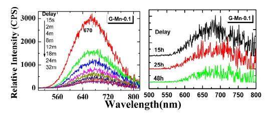
**Fig. 5.** Afterglow spectra of the glass sample G-Mn-0.1. The samples were pre-irradiated with an UV-254nm lamp for 5 min and measured at different delay times (15 seconds to 48hours) after removing the lamp.
