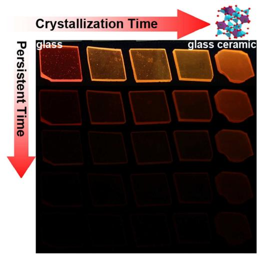
Red to near infrared ultralong lasting luminescence from Mn2+-doped sodium gallium aluminum germanate glasses and (Al,Ga)-albite glass-ceramics  $170 \times 170 \text{mm}$  (96 x 96 DPI)
