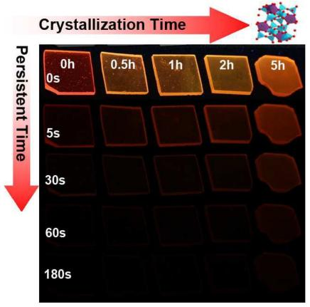
**Fig. 4.** Photographs of glass samples G-Mn-0.1 upon different crystallization time (0h~5h) and persistent time (0s~180s) after removal of excitation light of 254nm. Photos cannot be made for the longer persistent time because normal digital camera cannot recognize the weak signals.
