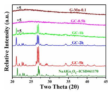
**Fig. 10.** XRD patterns of glass sample G-Mn-0.1 and glass-ceramic samples GC-0.5h, GC-1h, GC-2h and GC-5h. The simulated pattern of NaAlGe $_3$ O $_8$  (ICSD #61170) is shown for reference at the bottom of the figure.
