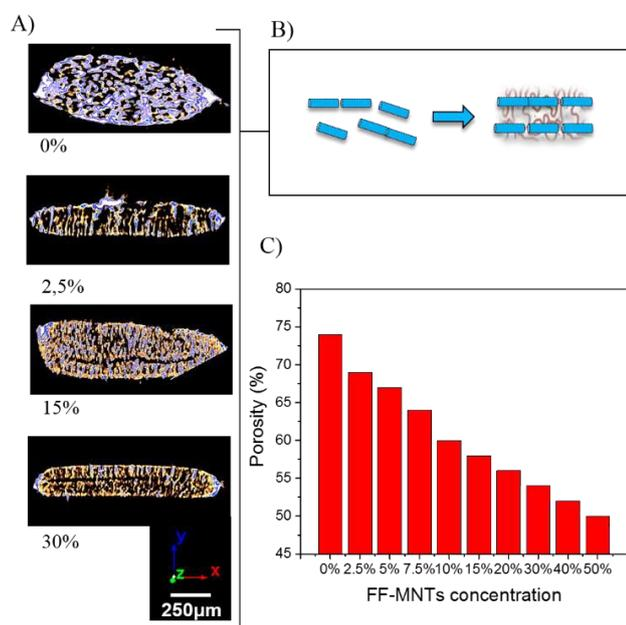
**Figure 4.** Microtomography analyses from FF-MNTs/PCL samples. (A) Representative slices showing the inner morphology of the membranes, exposing the porous network; (B) Schematic representation for the proposed organization framework where the presence of FF-MNTs induces local ordering on polymer network reinforcing its mechanical properties. The blue tubes denote the PCL fibers. (C) Porosity of the membranes obtained from the distribution of pores for ~500 slices.
