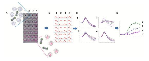
**Figure 1**: Overview of the approach used to allow direct measurement of carbohydrate-lectin interactions by monitoring a colourimetric change (red to blue) due to aggregation of glycoAuNPs bound to lectins (A) and the use of absorbance spectra (B and C) in the formation of binding curves (D).
