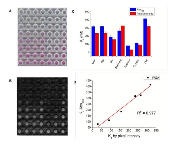
**Figure 3**: Direct optical analysis of lectin/glycan interaction. A) Scanned image of glycoAuNPs with a dilution series of WGA after 30 minutes incubation at 37 °C. B) Saturation image used for pixel intensity measurement (high intensity = red, low intensity = blue). C) Comparison of  $K_d$  calculated by  $Abs_{700}$  and pixel intensity. D) Correlation between  $K_d$  values determined by  $Abs_{700}$  and pixel intensity.
