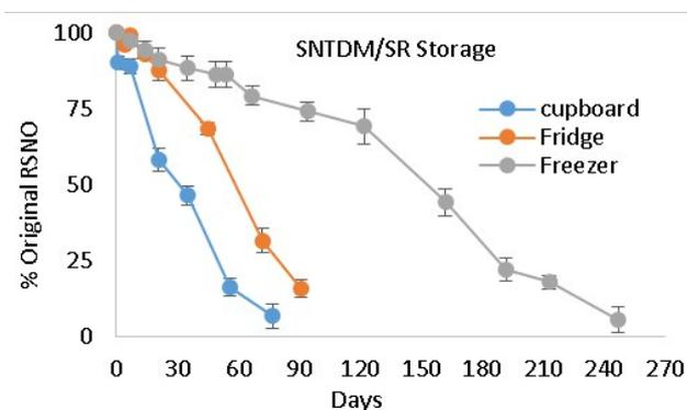
Fig. 7 SNTDM impregnated SR tubing stored in various environments
