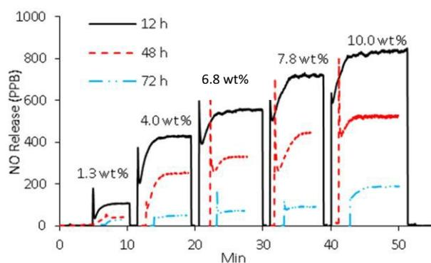
**Fig. 4** Initial NO release in parts per billion (ppb) for SR tubing impregnated with various wt% SNTDM (S.A. 0.42 cm<sup>2</sup>). SNTDM/SR adopts a steady-state flux quickly, taking less than 10 min.
