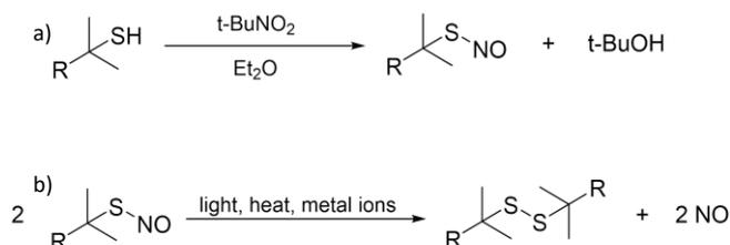
**Fig. 1** (a) Nitrosation of *tert*-dodecyl mercaptan (TDM) to yield *S*-nitroso-*tert*-dodecyl mercaptan (SNTDM). (b) Decomposition can be catalysed by light, heat, or metal ions such as Cu (I) to yield the disulfide and 2 equivalents of nitric oxide (NO). R=C<sub>9</sub>H<sub>19</sub> isomer.
