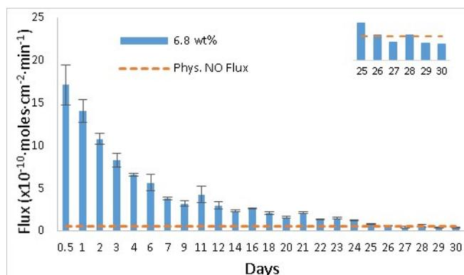
**Fig. 5** Long term NO flux for the 6.8wt % loaded SR tubing stored under physiological conditions (37 °C, PBS + EDTA buffer, in dark).
