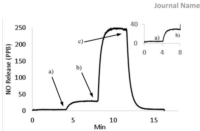
Fig. 6 SR tubing impregnated with 1.3 wt% SNTDM (S.A.  $0.42 \text{ cm}^2$ ) at  $22.5^\circ \text{C}$  in the dark, with a) fluorescent light, with b) fluorescent light and a broad spectrum halogen lamp, and again, in the c) dark.
