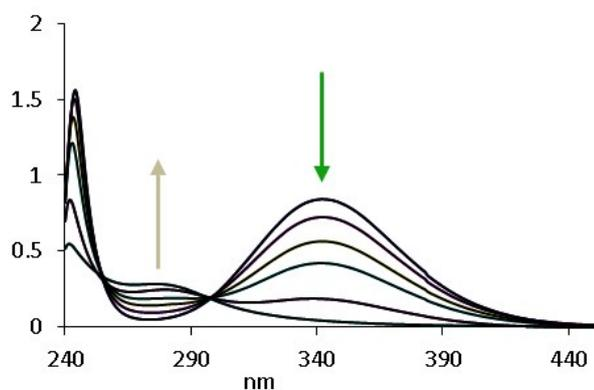
**Fig. 2** Spectra displaying the inverse relationship between SNTDM (341 nm) and DTDD (275 nm) absorbances during decomposition.
