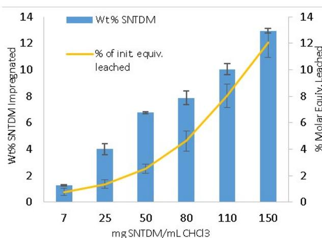
**Fig. 3** The soaking solutions' SNTDM concentration affects the amount of impregnation, which in turn relates to leaching. The reported leaching levels are the final cumulative concentrations corresponding to the SNTDM/SR tubing's NO release lifetime.
