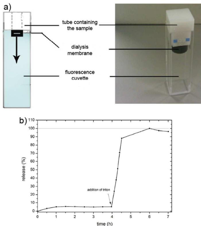
**Fig. 5** (a) Schematic presentation and photo of the release setup.<sup>31, 42</sup> (b) Release profile of calcein in SLB@MCS at 37 °C.
