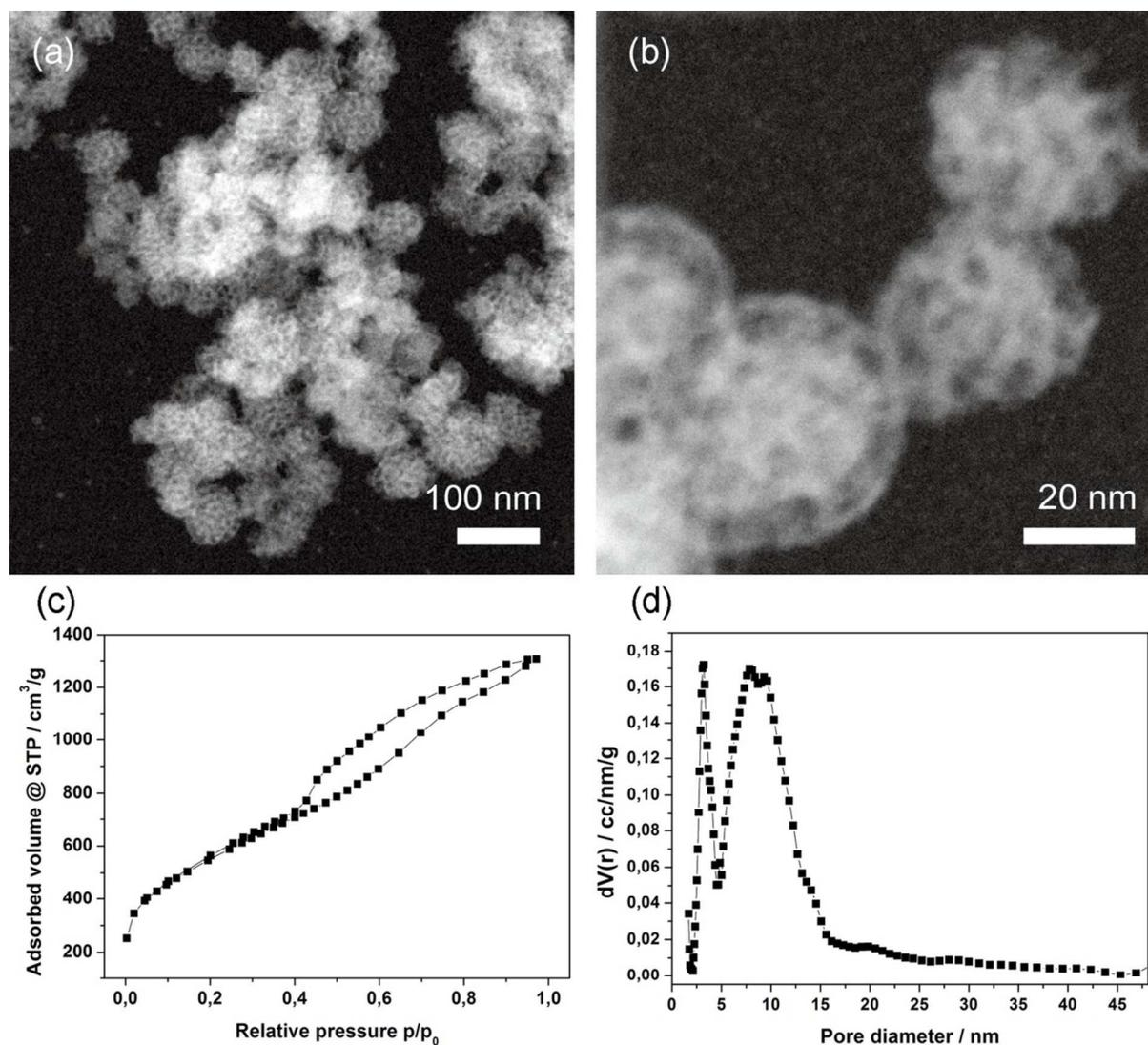
**Fig. 3** (a, b) STEM-HAADF images of MCS at different magnifications, obtained after HF treatment. Nitrogen sorption measurements reveal a type IV isotherm (c) and a bimodal pore size distribution (d).
