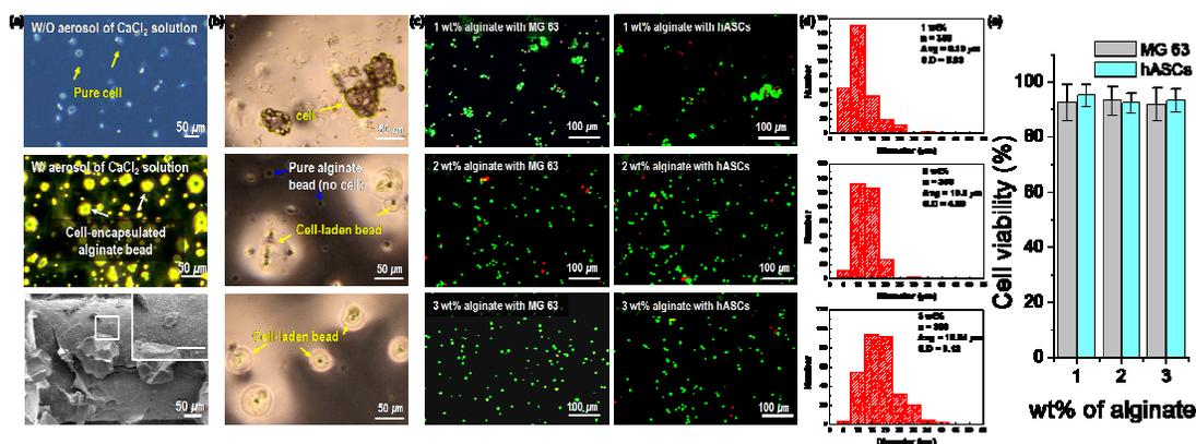
Figure 2. (a) Optical and SEM images of aerodynamically sprayed cell-laden alginate beads with and without an aerosol of  $\text{CaCl}_2$  solution during the process. (b) Optical and (c) fluorescence (live = green, dead = red) images of cell-laden alginate beads sprayed with three different alginate concentrations (1, 2, 3 wt%). (d) Diameter distribution of cell-laden alginate beads. (e) Cell viability of the cell-laden beads with three different alginate concentrations.
