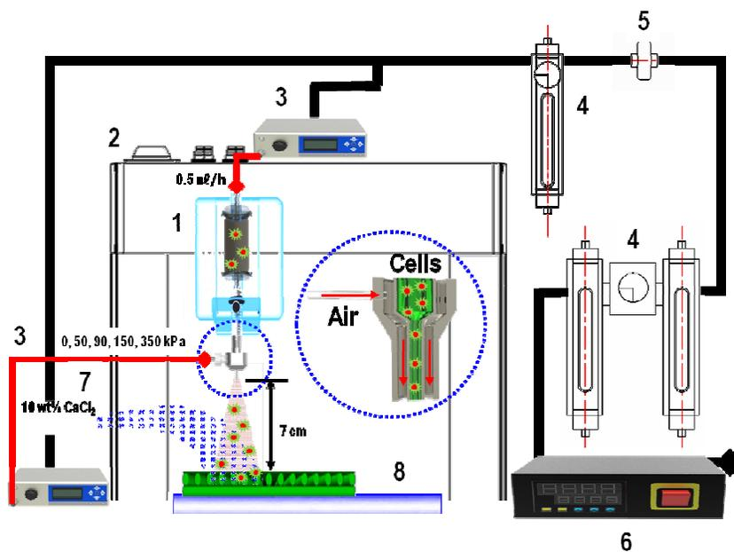
Figure 1. Scheme of the cell-spraying device: (1) a cell-laden alginate spraying system using a core-shell nozzle, (2) three-axis robot system, (3) a controller system for dispensing air, (4, 5, 6) filtering systems for air, (7) an aerosol system for CaCl<sub>2</sub> solution, and (8) a working stage.
