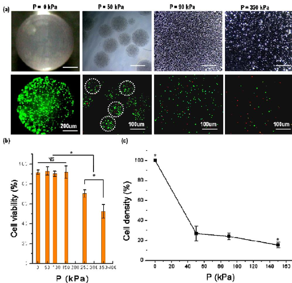
Figure 4. (a) Optical and fluorescence (live = green, dead = red) images of cell-laden alginate beads sprayed with various air pressures (0, 50, 90, and 350 kPa) in the shell nozzle. (b) Cell viability and (c) the relative density (%) of sprayed cell-laden alginate beads per the same collecting area.
