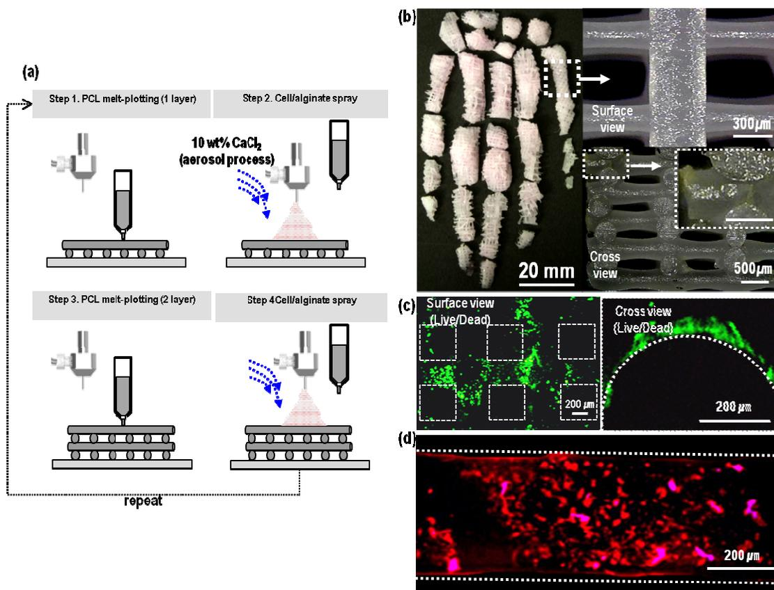
Figure 6. (a) Schematic description of hybrid scaffold fabrication. (b) An optical image showing the cell-laden hybrid scaffold. (c,d) Live and DAPI/phalloidin images of the hybrid scaffold after a 7-day culture period.
