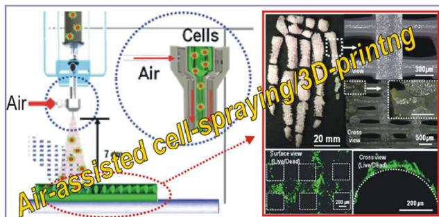
Here, the atomization process to obtain homogeneous cell-laden microbeads was proposed, and they were sprayed simultaneously onto the surface of a PCL mesh structure in a layer-by-layer manner to obtain the cell-laden hybrid structure.
