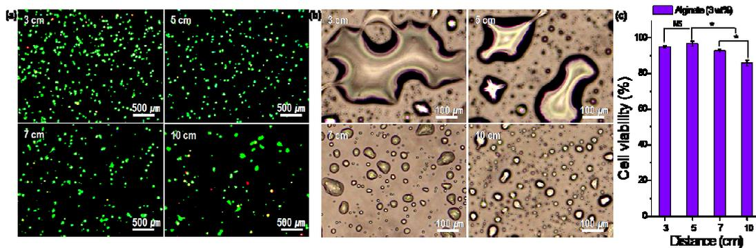
Figure 3. (a) Fluorescence (live = green, dead = red) images and (b) optical images of cell-laden alginate beads sprayed at four different distances (3 cm, 5 cm, 7 cm, and 10 cm) between the spraying nozzle and collector. (c) Cell viability of cell-laden beads fabricated at the various distances.
