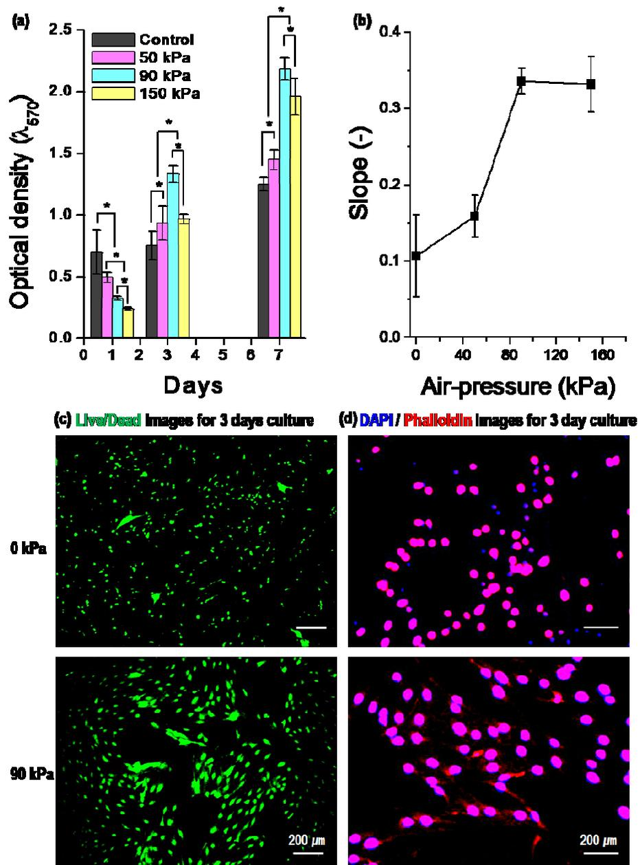
Figure 5. (a) Results of the MTT assay for the cell-laden alginate beads fabricated with several air pressures (0 [control], 50, 90, and 150 kPa) and (b) the slope of the MTT result describing the rate of cell proliferation. (c) Live/dead and (d) DAPI/phalloidin images of the cell-laden beads fabricated using 0 pressure (control) and 90 kPa.
