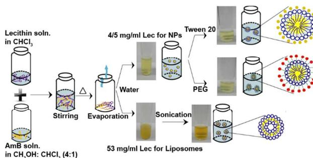
Fig. 1 Synthetic scheme for the formation of Lec-AmB NPs and liposomes.
