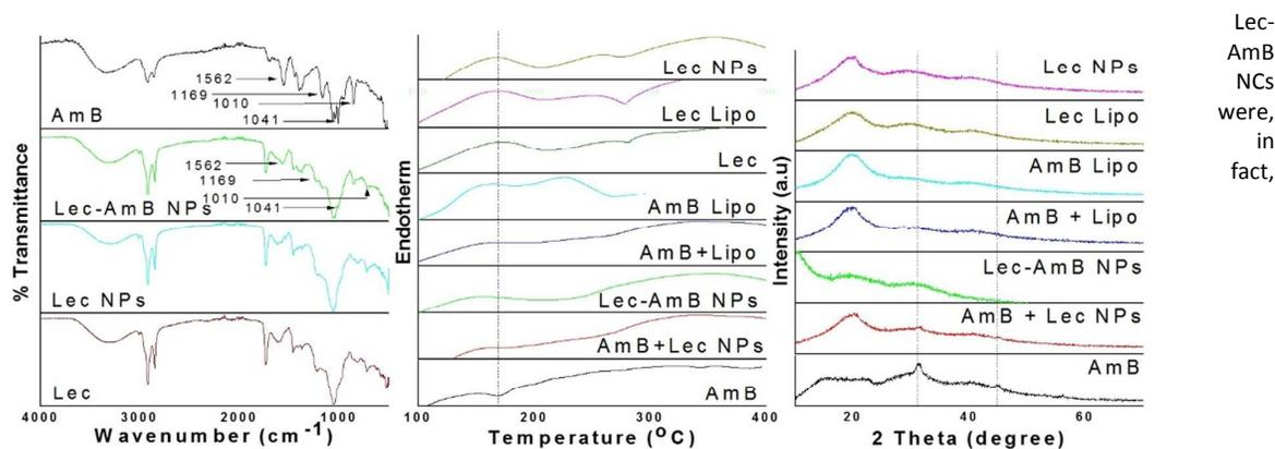
Fig. 4 XRD, DSC and FTIR results of AmB, Lecithin, empty Lec-NPs and Liposomes, Lec-AmB NPs and Liposomes and physical mixture of empty Lec-NPs and Liposomes with AmB.
