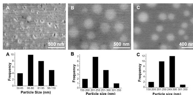
**Fig. 2** Scanning electron micrographs of AmB lecithin NPs, liposomes and their respective size distribution histograms. (A) AmB-Lec Liposomes, (B) AmB-Lec Tw NPs and (C) AmB-Lec PEG NPs.
