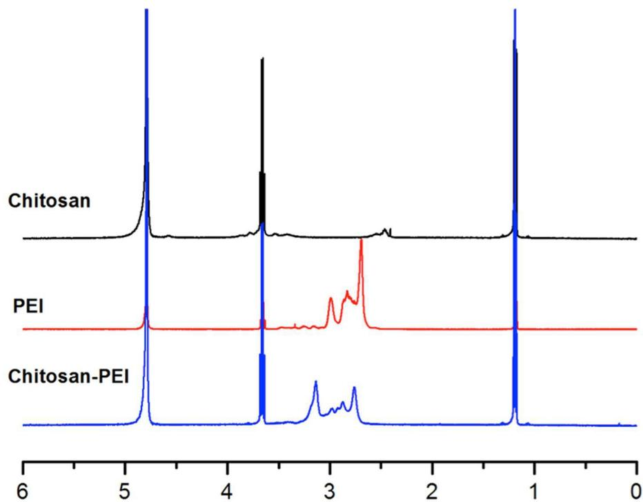
Figure 2. <sup>1</sup>H NMR spectra of chitosan, PEI, and chitosan-PEI copolymer.
