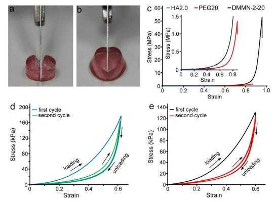
Fig. 6 (a) The PEG20 gel is easily sliced with a scalpel, while (b) the DMMN-2-20 gel can
