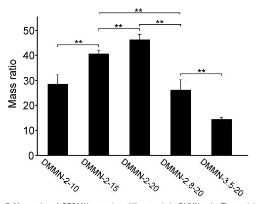
525 **Fig. 7** Mass ratios of PEG20K network to HA network in DMMN gels. The statistical significance is indicated with \*\* ( $p \le 0.01$ ).
