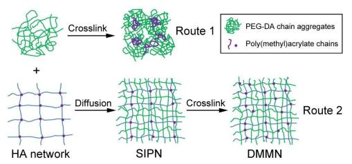
513 Fig. 5 Schematic fabrication process of PEG gel (Route 1) and DMMN gel (Route 2). SIPN
