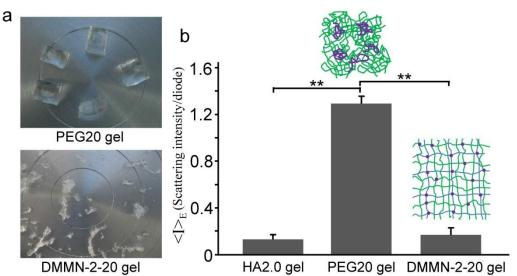
506 DMMN-2-20 gei HA2.0 gei PEG20 gei DMMN-2-20 gei 507 **Fig. 4** (a) Images of PEG20 and DMMN-2-20 gel after compression failure. (b)  $\langle I \rangle_E$  of HA2.0,
