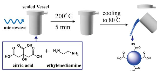
**Scheme 1** Schematic diagram for synthesizing CDs via microwave-assisted heating with controllable temperature.
