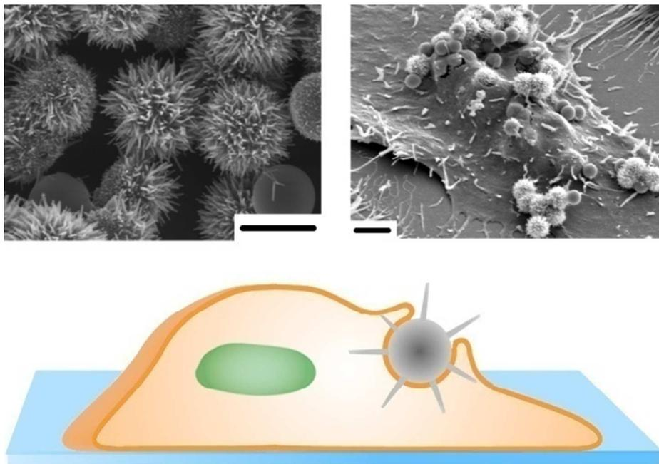
Synthesis of hierarchical “spiky” nanoparticles covered with stiff nanowires for biological cellular interface and engulfment.
