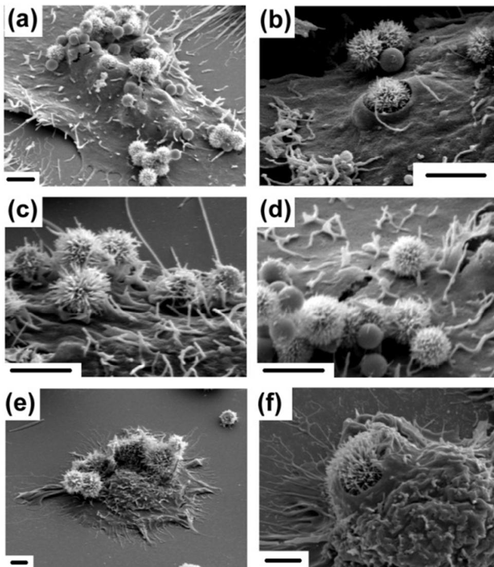
**Figure 3.** SEM images of spiky particle-cell interface. (a)-(d) Spiky particles were fabricated using 800 nm  $\text{SiO}_2$  nanospheres as the core. The spiky particles appear to be either internalized, partially engulfed, or resting on the cell surfaces. (e) and (f) Spiky particles were fabricated using larger  $\text{SiO}_2$  particle (2  $\mu\text{m}$ ) as the core. The spiky particles were engulfed by the cells. Scale bar: 2  $\mu\text{m}$ .
