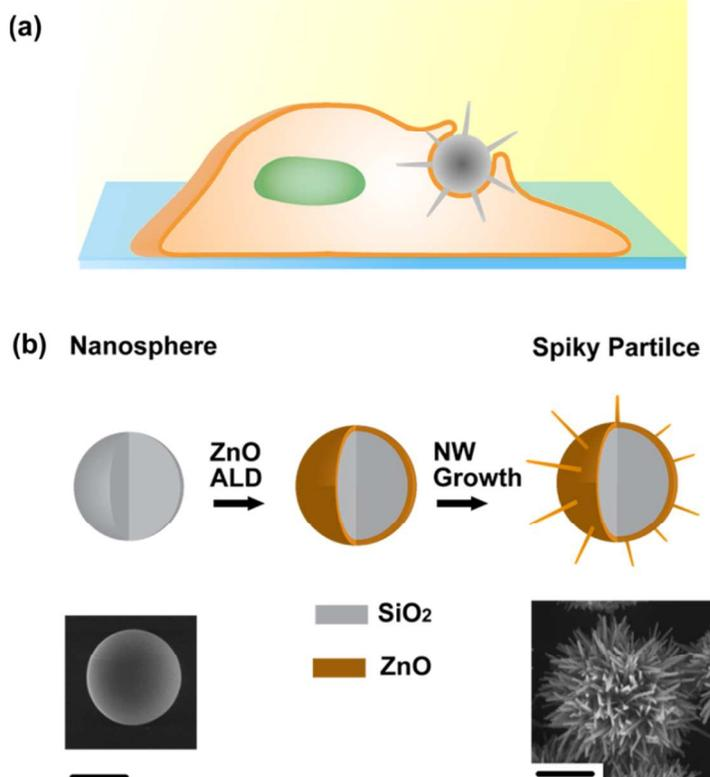
**Figure 1.** (a) Illustration of cell interfaces with spiky particle. (b) Illustration of spiky particle fabrication process. SiO<sub>2</sub> nanospheres were used as core particles. They were coated with 20-nm ZnO by ALD, and then ZnO NWs were grown on them to produce spiky particles. Scale bar: 500 nm.
