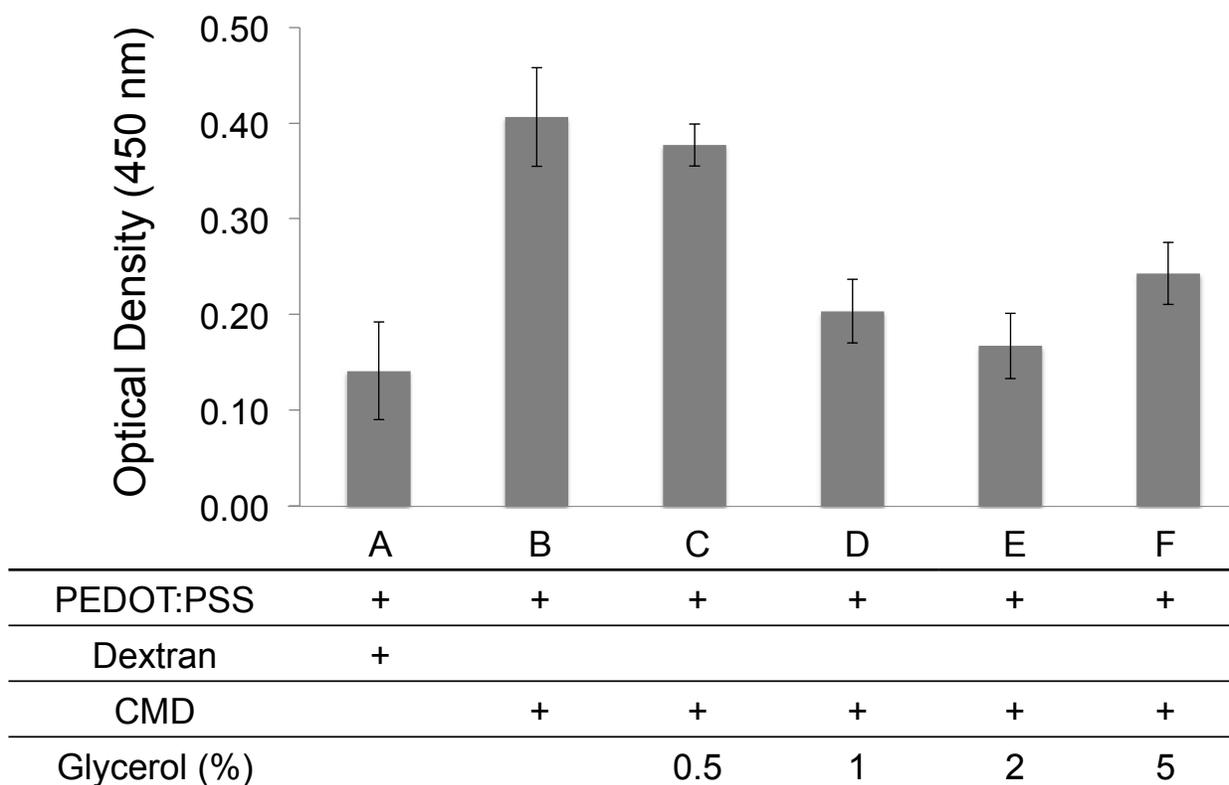
**Figure 5.** Stability of PEDOT:PSS films in PBS. PEDOT:PSS suspensions containing CMD (0.1% w/v), glycerol (1% v/v), with or without glycidoxypropyltrimethoxysilane (GOPS, 1% v/v) were spin-coated on pristine (conditions A and C) or GOPS-treated (condition B) glass surfaces. A profilometer was used to measure the thickness before and after immersion in phosphate buffered saline (PBS, 10 mM, pH 7.4).
