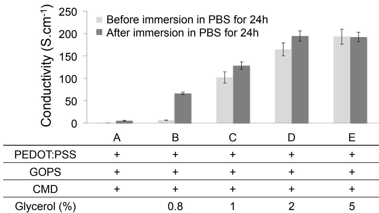
**Figure 7.** Impact of glycerol on the –COOH groups reactivity in GOPS-containing PEDOT:PSS films. Prior to the spin coating and the drying processes, PEDOT:PSS suspensions containing 0.1% w/v CMD and 1% v/v GOPS were mixed with glycerol (concentration ranging from 0 to 5% v/v).
