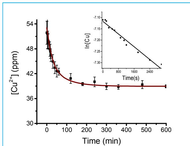
Fig. 3 Kinetics of copper removal from the aqueous solution by Au@D-PEN NPs. The inset shows the curve-fitting plot of a *pseudo* first order law.
