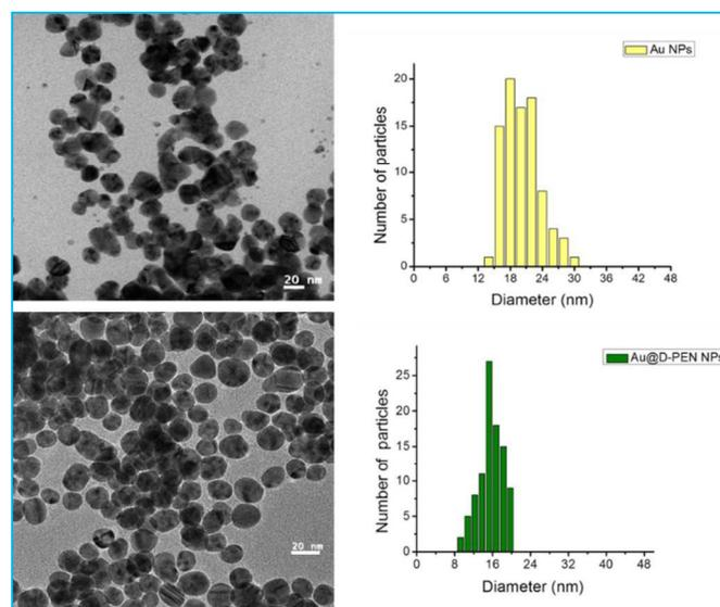
**Fig. 1** TEM images of as-prepared Au NPs (upper left) and Au@D-PEN NPs (lower left) and the histograms of the particle size distribution for NPs corresponding to each panel on the right mg/mL as determined by quantitative dispersability measurements.
