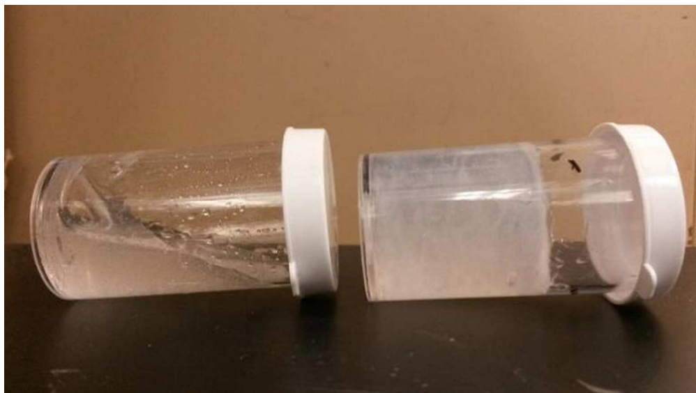
Figure 1: Suspension (left) and gel (right) states of alginate hydrogels 36x20mm (600 x 600 DPI)
