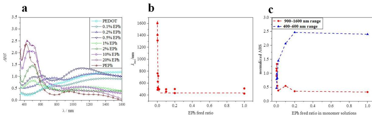
**Figure 4** (a) UV-vis-NIR absorption of the PEDOT-co-EPh copolymers; (b)  $\lambda_{\text{max}}$  versus composition; (c) normalized absorption in near-infrared (900-1600 nm) and visible (400-600 nm) wavelength range versus composition.
