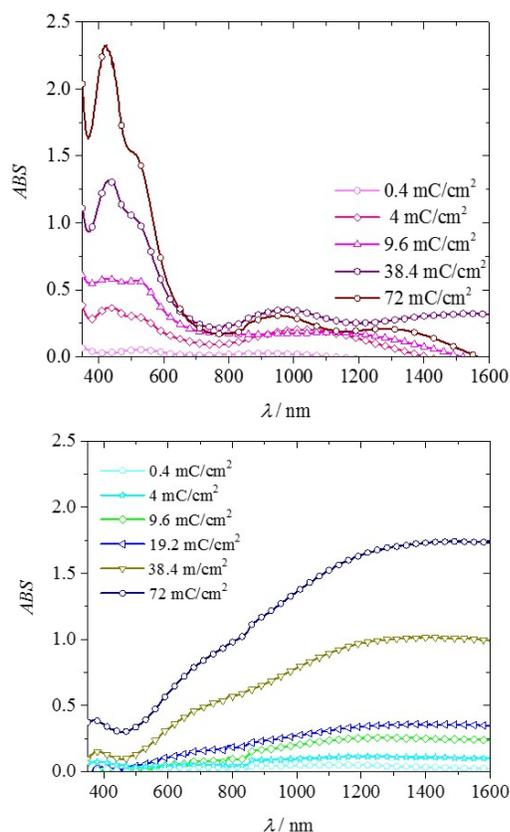
**Figure 5** UV-Vis-NIR spectra of polymers at different deposition charges. Top: PEPH; Bottom: PEDOT. The insert is
