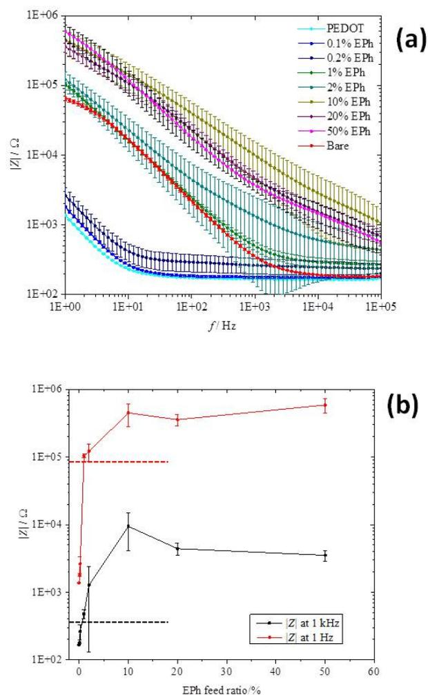
**Figure 7** (a) Impedance amplitude of PEDOT and PEDOT-co-EPh copolymers as a function of frequency; (b) impedance amplitude at 1 Hz and 1 kHz for the PEDOT-co-EPh copolymers as a function of EPH content; dashed lines indicate the impedance amplitude of bare Pt electrode at 1 Hz (red) and 1 kHz (black), respectively. (Deposition charge: 288  $\text{mC}/\text{cm}^2$ )
