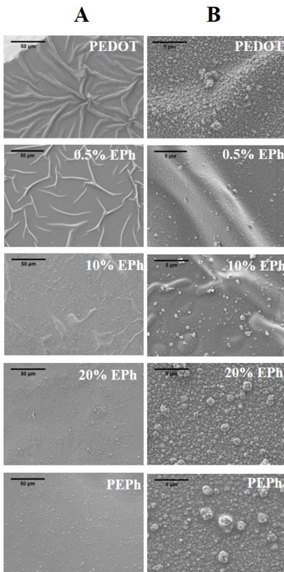
**Figure 6** SEM images of P(EDOT-co-EPh) films as a function of EPH feed ratio; A column: lower magnification (scale bar represents 50  $\mu\text{m}$ ); B column: higher magnification (scale bar represents 5  $\mu\text{m}$ )
