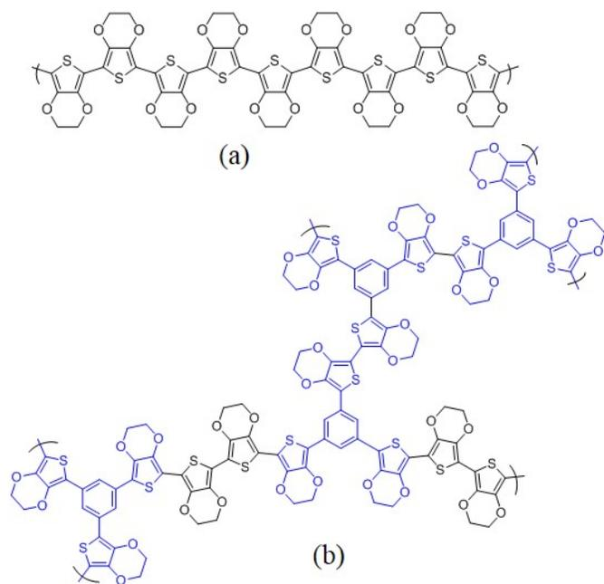
**Figure 1** (a) PEDOT and (b) Eph crosslinked PEDOT.
