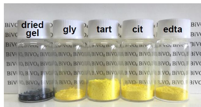
Fig. 3 Photographs of the dried gel obtained by dryness of the Bi(edta)+V(tart)-sol. and the AC-L samples obtained by dryness of the precursor solution Bi(edta)+V(L)-sol. (L = (a) gly, (b) tart, (c) cit or (d) edta) followed by calcination at 500°C in air.
