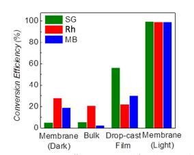
**Figure 4** Conversion efficiency measured after 2 hrs using three different types of  $g\text{-}C_3N_4$  (bulk  $g\text{-}C_3N_4$ , drop casted  $g\text{-}C_3N_4$  film and  $g\text{-}C_3N_4$  laminates obtained by filtration). A control experiment in the dark was also performed for the  $g\text{-}C_3N_4$  laminates to evaluate the adsorption ability of the membrane.
