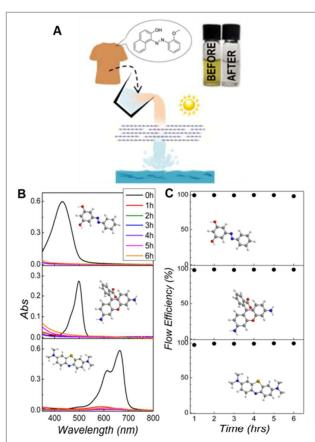
**Figure 3** (a) Schematic of the membrane-based continuous flux degradation of Sudan Orange G (SG) and pictures of the dispersions before and after treatment. b) Time-evolution of the UV-Vis spectra for all three dyes investigated: sudan orange G (SG), Rhodamine 110 (Rh) and methylene blue (MB). c) Flow efficiency measured for 6 hours for different organic pollutants.
