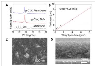
**Figure 2** a) X-ray diffraction pattern of melamine, g- $C_3N_4$  bulk and membrane; b) Thickness of g- $C_3N_4$  laminates as a function of the weight per area; in-plane (c) and cross section (d) SEM images of a g- $C_3N_4$  membrane.
