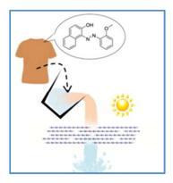
**Novel membrane photo-reactor based on 2D crystals**: the discovery of new materials is fundamental in developing novel and efficient membrane photo-catalytic reactors. We demonstrated that g-C3N4 nanosheets can be assembled in membranes permeable to water, which allow making low-cost, efficient, easy-to-produce self-catalytic photo-reactors for water treatment under visible light.
