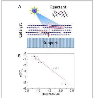
**Figure 5** a) Schematic of 2D-nanosheets based reactor for photo-degradation. b) Change in the concentration of SG after 2 hrs as a function of the laminate thickness.
