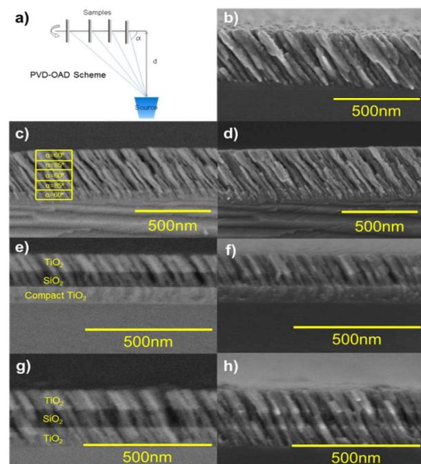
**Figure 2.** a) Schematic representation of the Physical Vapour Deposition at Oblique Angle (PVD-OAD) technique here employed to fabricate photonic crystal architectures. b) Cross sectional field effect scanning electron microscopy images (FE-SEM) using
