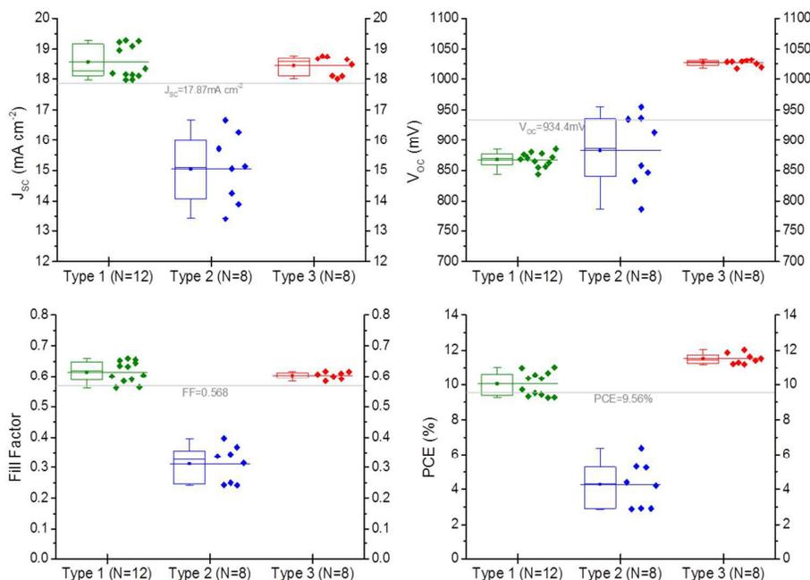
Figure 4. Box-whiskers plot which shows all the photovoltaic magnitudes for the different devices containing 1-DPC porous structures: PC1 (green), PC2 (blue) and PC3 (red). Grey lines represent the average values for each magnitude in the case of a reference  $\text{TiO}_2$  nanocolumnar photoanode. Dots at the right of the box mean the exact value of each sample.
