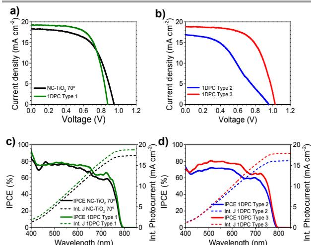
**Figure 3.** a) *J-V* characterization of the PSC containing TiO<sub>2</sub> tilted nanocolumns at  $\alpha=70^\circ$  (black) and PC1 (green). b) *J-V* characterization of the PSC containing PC2 (blue) and PC3 (red). c) *IPCE* spectra for the PSC with TiO<sub>2</sub> tilted nanocolumns at  $\alpha=70^\circ$  (black) and PC1 (green). d) *IPCE* spectra for the PSC with PC2 (blue) and PC3 (red).
