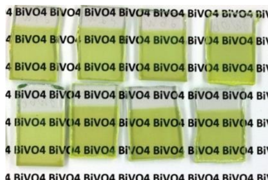
Fig. 5 Photograph showing the optical transparency of multilayer \text{BiVO}_4 electrodes (8 layers) prepared under the same conditions by spin-coating and after a final heat-treatment in air at 460°C.
