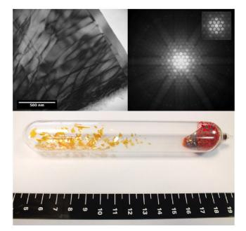
Fig. 2 Top left - Bright field transmission electron microscopy of an  $SnS_2$  platelet, image near the [0001] zone axis. Top right - Selected area diffraction pattern near the [0001] zone axis and, inset, the convergent beam electron diffraction for the same sample. Bottom centre - Macroscopic single crystals synthesised from the CVT method, with the scale in centimetres.
