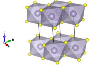
Fig. 1 Ground state (2H) structure of  $SnS_2$  showing the 2-dimensional bonded plane of edge-sharing bonded octahedra and the conventional unit cell.
