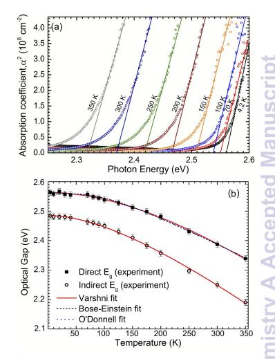
**Fig. 5** (a) Optical absorption spectra as a function of temperature and (b) corresponding direct (closed squares) and indirect (open circles) band gaps for the same single crystal of tin disulfide. Also shown are Varshni, Bose-Einstein and O'Donnell fits to the direct band gaps and a Varshni fit to the indirect band gap.
