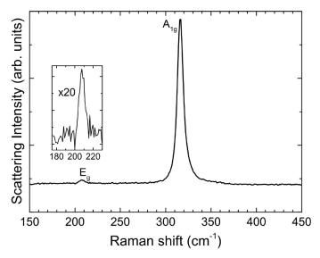
Fig. 3 Raman spectrum from SnS<sub>2</sub>, with A<sub>1g</sub> and E<sub>g</sub> modes indicative of the 2H polytype. The inset shows a 20 times magnification of the E<sub>g</sub> mode.
