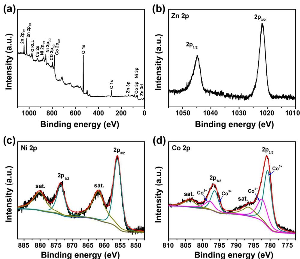
Fig. 5 XPS spectra for the  $\text{ZnCo}_2\text{O}_4@Ni_x\text{Co}_{2x}(\text{OH})_{6x}$  core/shell NWAs: survey spectrum (a) and high-resolution spectra of Zn 2p (b), Ni 2p (c) and Co 2p (d).
