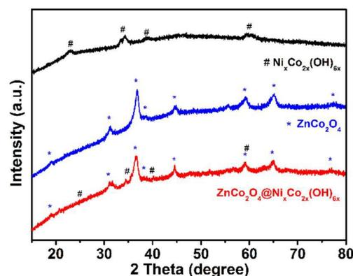
Fig. 4 XRD patterns of the  $\text{ZnCo}_2\text{O}_4$ ,  $(\text{Ni}_x\text{Co}_{2-x})(\text{OH})_{6x}$  and  $\text{ZnCo}_2\text{O}_4@(\text{Ni}_x\text{Co}_{2-x})(\text{OH})_{6x}$  nanostructures scratched from Ni foam.
