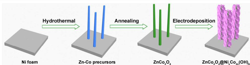
Fig. 1 Schematic illustration of the construction process of hierarchical ZnCo<sub>2</sub>O<sub>4</sub>@Ni<sub>x</sub>Co<sub>2x</sub>(OH)<sub>6x</sub> core/shell NWAs on Ni foam.
