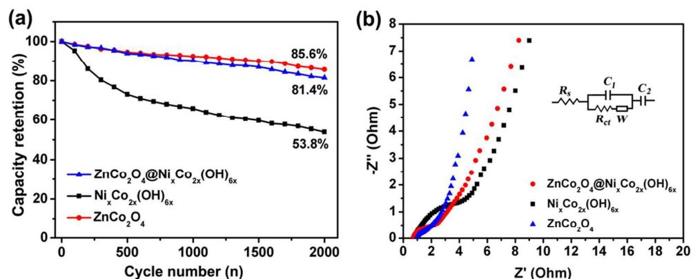
Fig. 7 (a) Cycling performance of the prepared  $\text{ZnCo}_2\text{O}_4@\text{Ni}_x\text{Co}_{2x}(\text{OH})_{6x}$ ,  $\text{Ni}_x\text{Co}_{2x}(\text{OH})_{6x}$  and  $\text{ZnCo}_2\text{O}_4$  electrodes during 2000 cycles at  $20 \text{ mA cm}^{-2}$ . (b) Nyquist plots of  $\text{ZnCo}_2\text{O}_4@\text{Ni}_x\text{Co}_{2x}(\text{OH})_{6x}$ ,  $\text{Ni}_x\text{Co}_{2x}(\text{OH})_{6x}$  and  $\text{ZnCo}_2\text{O}_4$  electrodes.
