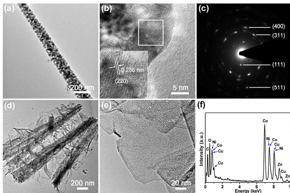
Fig. 3 TEM image (a), HRTEM image (b) and SAED pattern (c) of the  $\text{ZnCo}_2\text{O}_4$  nanowire. TEM images (d and e) and EDX spectrum (f) of the  $\text{ZnCo}_2\text{O}_4@(\text{Ni}_x\text{Co}_{2-x})(\text{OH})_{6x}$  NWAs.
