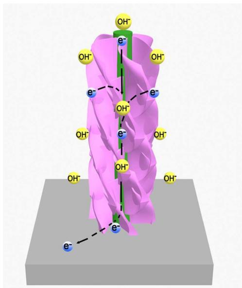
Fig. 8 Schematic illustration of the advantages of the hierarchical  $\text{ZnCo}_2\text{O}_4@\text{Ni}_x\text{Co}_{2x}(\text{OH})_{6x}$  NWAs
