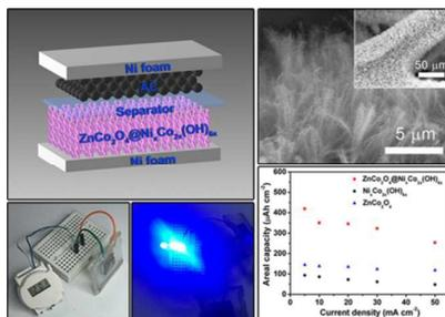
Hierarchical  $\text{ZnCo}_2\text{O}_4@\text{Ni}_x\text{Co}_{2x}(\text{OH})_{6x}$  core/shell nanowire arrays have been successfully constructed for hybrid supercapacitors with outstanding performance.
