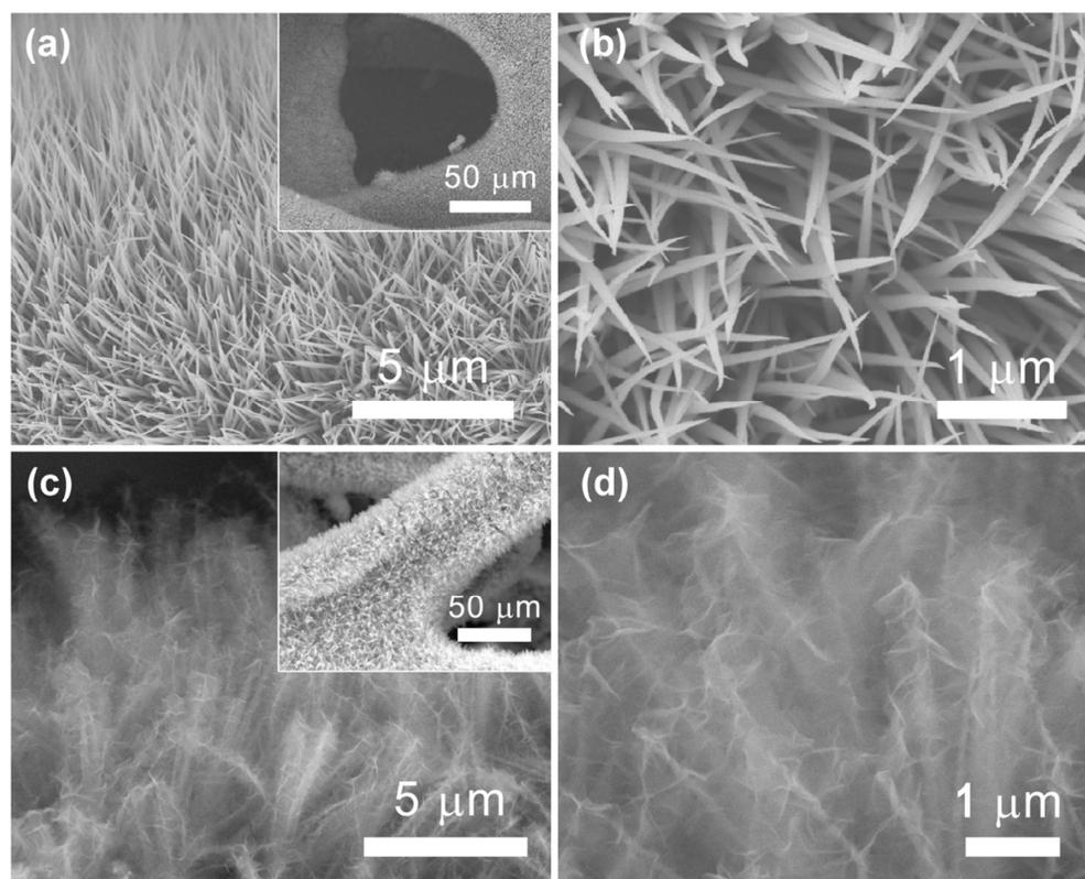
Fig. 2 SEM images of  $\text{ZnCo}_2\text{O}_4$  NWAs (a and b) and  $\text{ZnCo}_2\text{O}_4@ \text{Ni}_x\text{Co}_{2-x}(\text{OH})_{6x}$  NWAs (c and d) on Ni foam at different magnifications.
