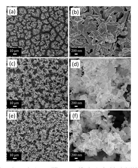
Fig.6. SEM surface micrographs (at two different magnifications) of calcined (950°C for 8 h in air)  $La_4Ni_3O_{10-\delta}$  films obtained by ESD at deposition temperatures of: (a), (b) 300 °C; (c), (d) 350 °C; (e), (f) 400 °C with a solution concentration of 0.02 M for a nozzle to substrate distance of 50 mm and a flow rate of 1.5 mL.h<sup>-1</sup> and after deposition time of 3 h.
