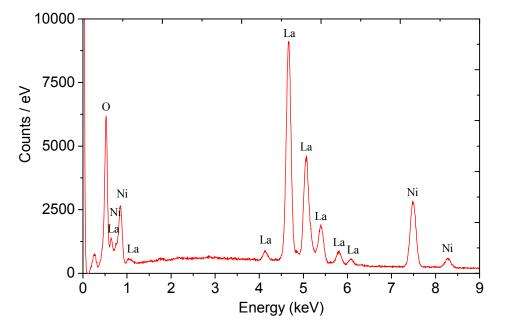
Fig.2. Typical EDX spectrum of the La<sub>4</sub>Ni<sub>3</sub>O<sub>10-δ</sub> film calcined at 950 °C for 8 h in air
