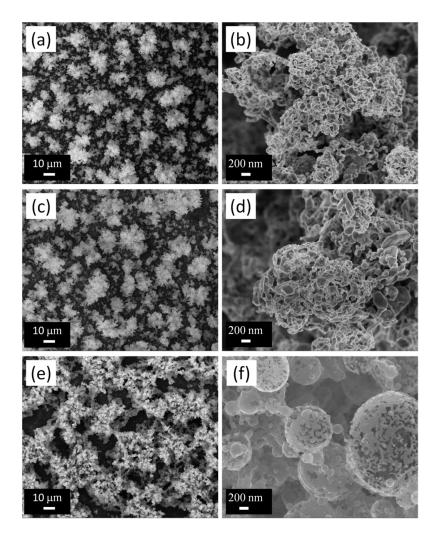
Fig.4. SEM surface micrographs (at 2 different magnifications) of calcined (950 °C for 8 h in air)  $La_4Ni_3O_{10-\delta}$  ESD films obtained with a solution concentration of (a), (b) 0.005 M; (c) (d) 0.01 M; (e), (f) 0.02 M, using pure EtOH at T=350 °C for a nozzle to substrate distance of 50 mm and a flow rate of 1.5 mL.h<sup>-1</sup> and after deposition time of 3 h.
