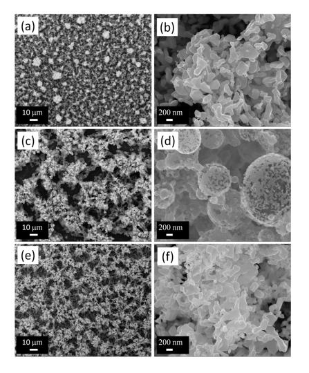
Fig. 5. SEM surface micrographs (at 2 different magnifications) of calcined (950 °C for 8 h in air)  $La_4Ni_3O_{10-\delta}$  ESD films obtained with solution of (a), (b)  $S_A$ : EtOH + BC (1:2); (c), (d)  $S_D$ : EtOH; (e), (f)  $S_E$ : EtOH +  $H_2O(1:2)$  with a solution concentration of 0.02 M at T=350 °C for a nozzle to substrate distance of 50 mm and a flow rate of 1.5 mL.h<sup>-1</sup> and after deposition time of 3 h.
