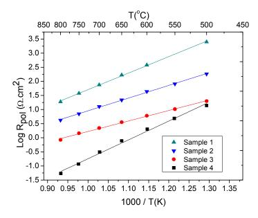
Fig. 11. Arrhenius plot of the  $R_{pol}$  in air for La<sub>4</sub>Ni<sub>3</sub>O<sub>10- $\delta$ </sub> electrodes (OCP conditions) on CGO electrolyte,(a) sample 1, isolated cauliflower (b) sample 2, connected round agglomerates (c) sample 3, 3-D coral type (d) sample 4, double layer cathode ( 3-D coral type + SP).
