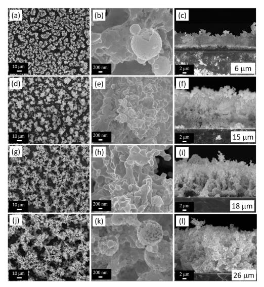
Fig. 3. SEM micrographs of the calcined (950°C for 8 h in air) ESD films using EtOH and 0.02 M salt concentration at T=350 °C, for a distance nozzle to substrate of 50 mm and a flow rate of 1.5 mL.h<sup>-1</sup> after deposition time of: 0.5 h (a, b) surface, (c) cross section; 1.5 h (d, e) surface, (f) cross section; 2 h (g, h) surface, (i) cross section; 3 h (j, k) surface, (l) cross section.
