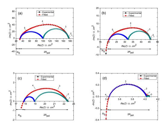
Fig. 9.Nyquist plots for the La<sub>4</sub>Ni<sub>3</sub>O<sub>10- $\delta$ </sub>/CGO/La<sub>4</sub>Ni<sub>3</sub>O<sub>10- $\delta$ </sub> cells with different microstructure recorded in air at 700 °C in OCP conditions: (a) sample 1 (b) sample 2 (c) sample 3 (d) sample 4. The numbers over the diagram indicate the logarithm of the measuring frequency.
