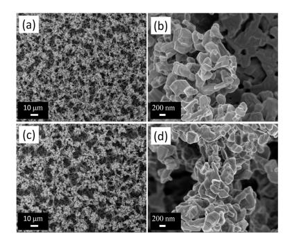
Fig. 7. SEM surface micrographs (at 2 different magnifications) of the calcined (950°C for 8 h in air)  $La_4Ni_3O_{10-\delta}$  films obtained at a deposition temperature of 350 °C, a deposition time of 3 h, a flow rate of 1.5 mL.h<sup>-1</sup> and a nozzle to substrate distance of: (a), (b) 30 mm; (c), (d) 50 mm with a S<sub>E</sub> solution of concentration 0.02 M.
