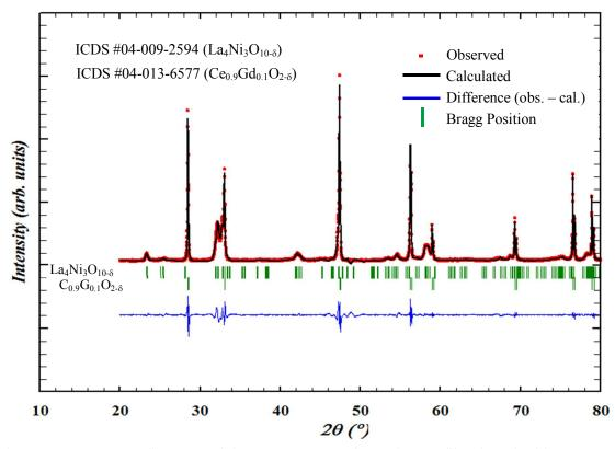
Fig. 1. FULLPROF refinement of the XRD pattern of La<sub>4</sub>Ni<sub>3</sub>O<sub>10- $\delta$ </sub> film deposited by ESD at 350 °C on a CGO substrate and after calcination at 950 °C/8 h + 1100 °C/6 h in air.
