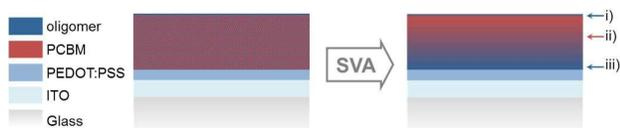
**Fig. 10** Scheme of the vertical configuration of the oligomer **2:PC<sub>61</sub>** or **71BM** solar cells. For the solvent-vapor annealed sample three regions are marked: i) oligomer-enriched surface, ii) sub-surface region with decreased concentration of oligomer, iii) a slightly oligomer-enriched region up to the bottom interface.
