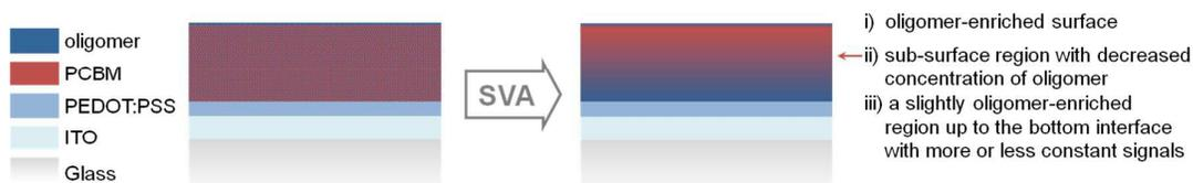
**Solvent vapor annealing (SVA)** can strongly influence the morphology of oligomer:fullerene – based organic solar cells: while for oligomer **1** with alkyl chains at the “outer” positions only crystallinity and domain size are increased, for oligomer **2** with alkyl chains at the more sterically hindered “inner” positions additionally a vertical gradient is formed after SVA.
