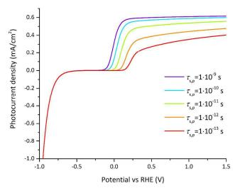
Figure 8 Photocurrent-voltage curves for varying hole surface lifetimes for the reference case (parameters indicated in Table 1 and 2). For large hole surface lifetimes (above 0.1 to 1 ns), surface recombination is negligible at large applied potentials. For small hole surface lifetimes (around 1 ps), the photocurrent is still affected by surface recombination at large potentials.
