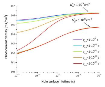
Figure 9 Photocurrent density at 1.23V vs RHE as a function of the hole surface lifetime for various electron lifetimes ( $\tau_{s,n}$ = 10<sup>-9</sup>,10<sup>-10</sup>,10<sup>-11</sup>,10<sup>-12</sup>,10<sup>-13</sup>s) and two doping concentrations ( $N_D^+$ =10<sup>16</sup> cm<sup>-3</sup> and  $N_D^+$ =10<sup>18</sup> cm<sup>-3</sup>).
