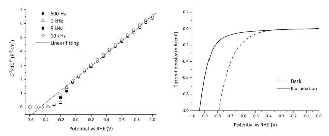
Figure 5 a) Mott-Schottky plot for four frequencies (500 Hz, 1 kHz, 5 kHz, 10 kHz) of a  $1\mu$ m-thick nid-GaN sample immersed in 1M H<sub>2</sub>SO<sub>4</sub> electrolyte under dark. b) Experimental dark current density (dashed line) and photocurrent density (solid line) vs RHE.
