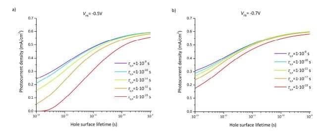
Figure 11 Photocurrent density at 0.3V vs RHE as a function of the hole surface lifetime for various electron lifetimes ( $\tau_{s,n}$  = 10<sup>-9</sup>,10<sup>-10</sup>,10<sup>-11</sup>,10<sup>-12</sup>,10<sup>-13</sup> s) and two flatband potentials: a)  $V_{FB}$  = -0.5V vs RHE, and b)  $V_{FB}$  = -0.7V vs RHE.
