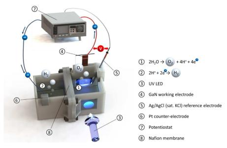
Figure 4 Scheme of the experimental PEC water-splitting test cell connected to the potentiostat. The UV LED illuminates the working electrode through air, quartz glass, and electrolyte.
