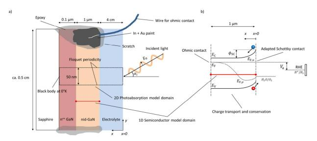
Figure 1 a) Scheme of the model domain (not to scale) of the photoanode (GaN) immersed in electrolyte including the 2D EMW propagation model domain (dotted) and boundary conditions, and the 1D semiconductor model domain (red line). b) Detailed 1D semiconductor model domain and boundary conditions.  $E_{\rm C}$  and  $E_{\rm V}$  are
