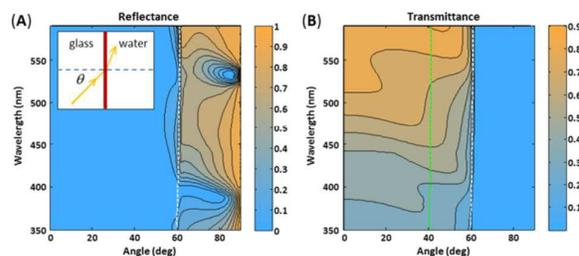
Fig. 5: Calculated reflectance (A) and transmittance (B) for a glass/FTO/SnO<sub>2</sub>/hematite/water stack illuminated from the glass side. The calculation domain is shown in the inset: The light ray, marked in orange, propagates at an angle  $\theta$  from the glass to the water via the FTO/SnO<sub>2</sub>/hematite stack that is shown in red.
