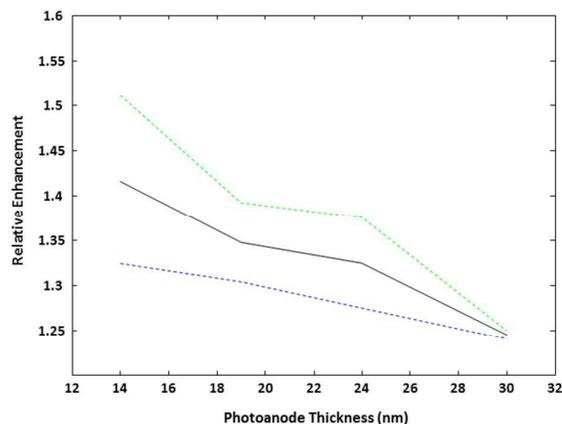
Fig. 8: Predicted photocurrent enhancement (relative to specular back reflector) without edge losses (solid black line) and measured photocurrent enhancement (dashed blue line) as a function of the hematite film thickness.
