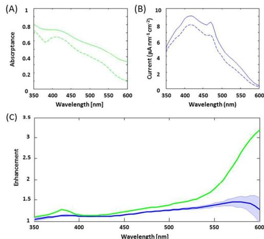
Fig. 6: Absorbance (A), plateau photocurrent (B) and relative enhancement spectra (C) obtained for the 19 nm thick hematite photoanode. Green and blue curves indicate absorbance and plateau photocurrent spectra, respectively, whereas solid and dashed lines correspond to results obtained with the Lambertian and specular back reflectors, respectively. The shaded region in panel C corresponds to the measurement errors.
