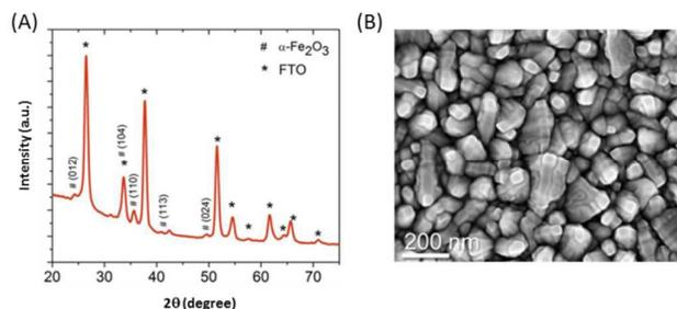
Fig. 2. Typical X-ray diffractogram (A) and high resolution scanning electron micrograph (B) of the thin film hematite photoanodes. Reproduced with permission from Ref. 25 (Cambridge University Press, 2015).
