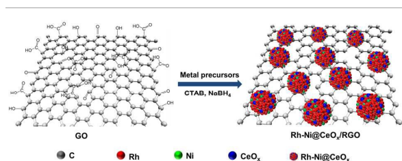
Scheme 1 Schematic illustration of preparation of the \text{RhNi}@/\text{CeO}_x/\text{rGO} NCs.
