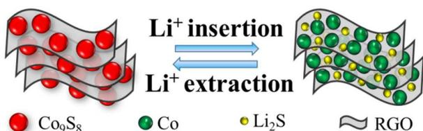
**Scheme. 2** The Schematic illustration of Li<sup>+</sup> insertion/extraction processes of RGO/Co<sub>9</sub>S<sub>8</sub> nanocomposite.
