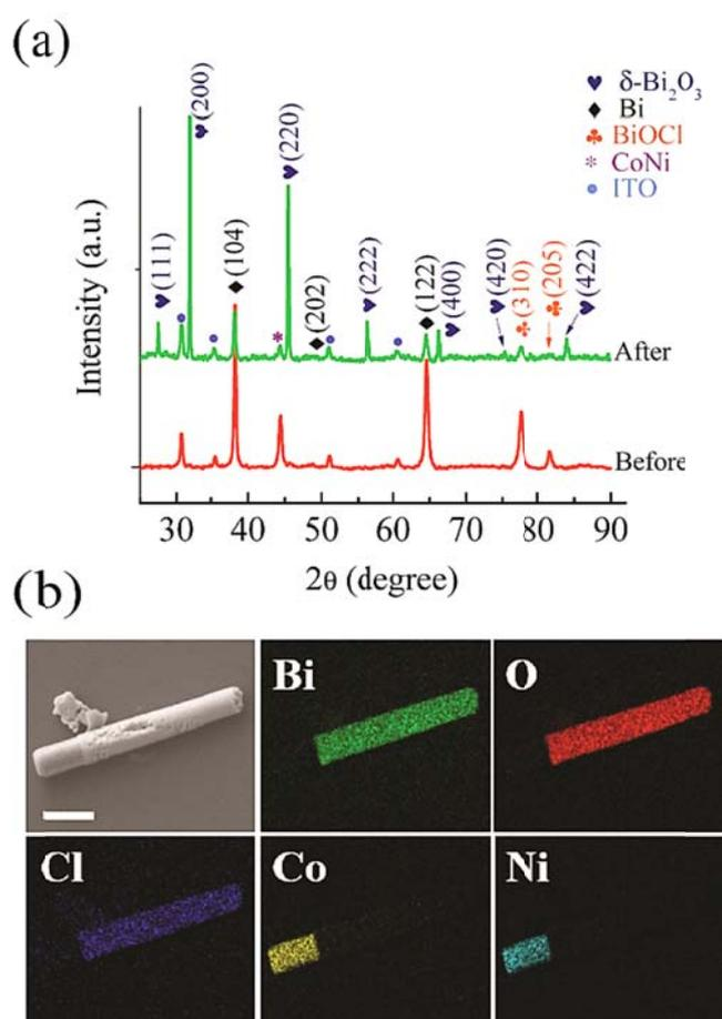
**Fig. 2** Structural characterization of hybrid micropillars. (a) XRD patterns of hybrid micropillars before and after exposure to water under UV light for 6 hours; (b) EDX mapping showing distribution of elements in an exposed hybrid micropillar (scale bar 2  $\mu\text{m}$ ).
