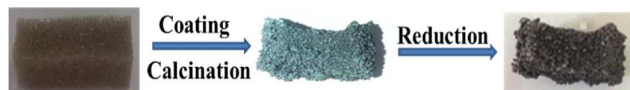
Fig. 1 Optical photos of the pure sponge, the sponge saturated precursors after calcination, and the black bulky sponge-shaped MoP (3D MoP).
