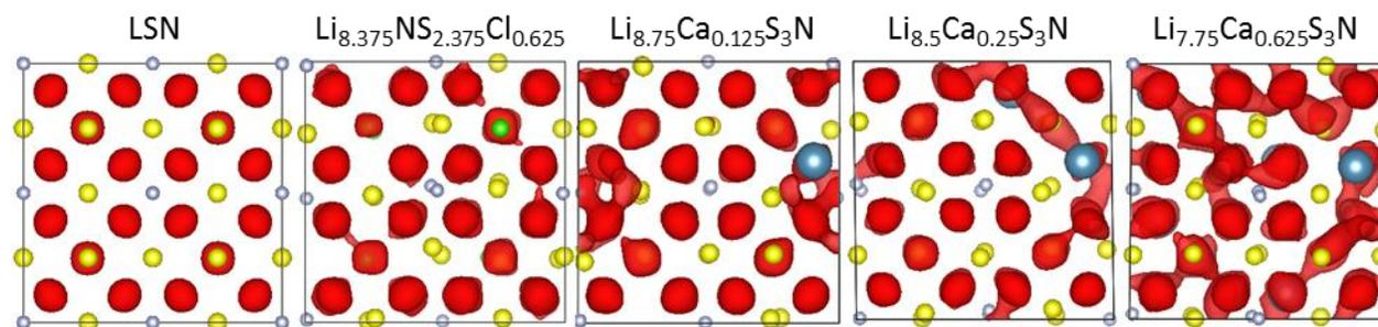
Figure 7: Isosurfaces of the ionic probability density determined from 800 K AIMD simulations.
