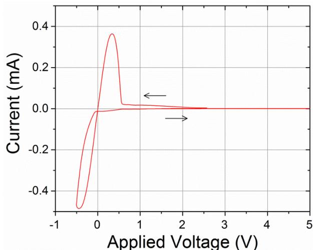
Figure 3: CV performed with a  $10 \text{ mV s}^{-1}$  scan rate. Li plating and stripping occurs, a small reduction peak is evident at about 0.5 V, but no further reaction is seen out to 5 V.
