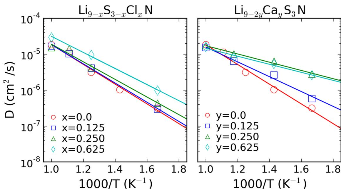
Figure 6: AIMD simulation results; left, Cl- and; right, Ca-substituted LSN. The Cl has limited effect on diffusivity while Ca-substitution beyond  $y = 0.25$  shows a rapid diffusivity and little change with further substitution.
