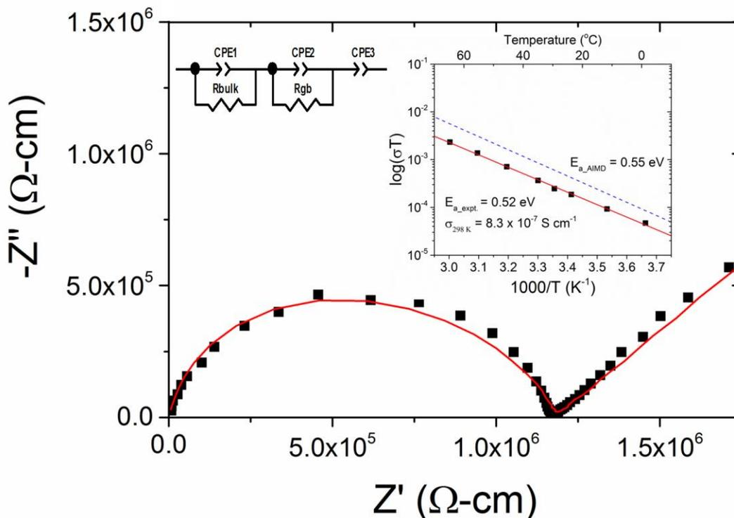
Figure 4: Nyquist plot of the EIS results at  $25^{\circ}\text{C}$ . The conductivity was extracted from the inset equivalent circuit. Results from other temperatures are plotted as an Arrhenius plot in the inset; the blue dashed line is AIMD simulation results for comparison.
