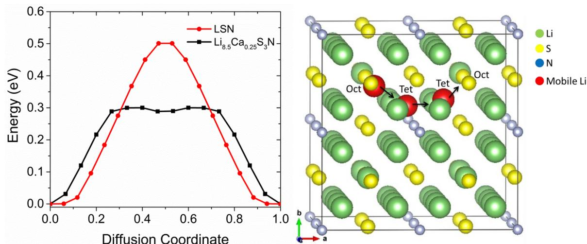
Figure 5: (left) Calculated NEB barrier for vacancy migration along oct-tet-tet-oct pathway with and without Ca. (right) Oct.-tet.-tet.-oct. migration pathway identified from NEB calculations. A coordinated three lithium movement is required.
