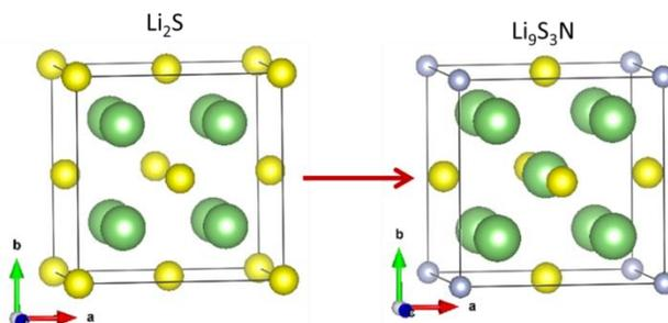
Figure 1: LSN is formed by substituting one S site in  $\text{Li}_2\text{S}$  with N and charge compensating with a Li at the 6 sulfur coordinated octahedral site; LSN has an anti-fluorite crystal structure with an FCC anion sublattice.
