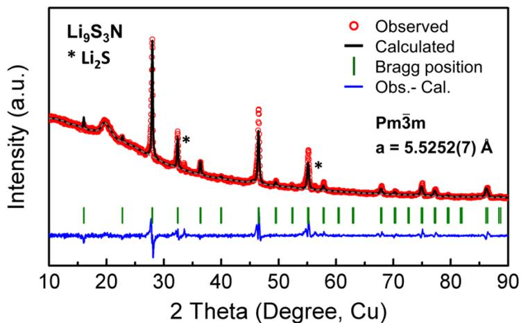
Figure 2: Rietveld refined XRD pattern obtained from  $\text{Li}_9\text{S}_3\text{N}$ . Fitting agreement indices are  $R_p = 4.69$ ,  $R_{wp} = 7.40$ , and  $\chi^2 = 9.65$  (Pseudo-Voigt fit).
