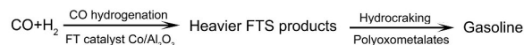
Scheme 1 The reaction mechanism of bifunctional catalyst consist of FTS catalyst and polyoxometalates
