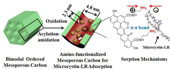
Amino-functionalized ordered mesoporous carbons were prepared with a high surface area and high-density amino groups, exhibiting preeminent static and dynamic adsorption capabilities (580 and 334 mg/g respectively) for Microcystin-LR removal.
