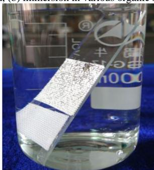
**Figure 6.** Immersion of the E-PET-S-F (upper) and pristine (lower) fabric stuck on glass into water.
