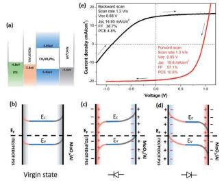
**Fig. 8** (a) Ideal energy-level diagram of ITO/PEDOT:PSS/MAPbl<sub>3</sub>/MoO<sub>3</sub>/Al heterojunction. Schematic energy band alignments of device in (b) virgin state (c) positively poled state (positive voltage is applied to Al), and (d) negatively poled state (positive voltage is applied to Al). Interface charge and screen charge are represented by red and black signs, respectively. Reproduced from ref. 26, copyright 2015, RSC.
