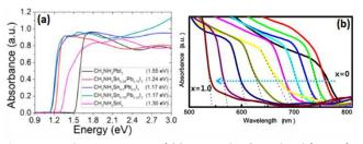
Fig. 3 UV-vis absorption spectra of (a)  $MASn_{1,x}Pb_xI_3$  (reproduced from ref. 84, copyright 2014, ACS) and (b)  $MAPb(I_{1,x}Br_x)_3$  (reproduced from ref. 85, copyright 2013, ACS).
