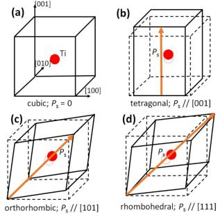
**Fig. 9** Schematics showing the structural distortion and the Ti displacement in four BaTiO<sub>3</sub> phases (a) cubic (reference), (b) tetragonal, (c) orthorhombic, and (d) rhombohedral. The spontaneous polarization orientations are indicated by brown arrows.
