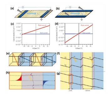
**Fig. 13** Schematics showing the orientation of electrodes (a) parallel and (b) perpendicular to domain walls. Corresponding I-V measurements of devices with (c) parallel and (b) perpendicular electrode configurations. (e) Schematic of 71° domain walls of BFO. Corresponding band diagrams (f) in the dark and (g) under illumination. (h) Detailed picture showing the build-up of photoexcited charge carriers near domain walls. Reproduced from ref. 33, Copyright 2010, Nature Publishing Group.
