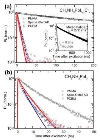
**Fig. 6** Time-resolved PL measurements of the (a) MAPbl<sub>3-x</sub>Cl<sub>x</sub> and (b) MAPbl<sub>3</sub> with PCBM (electron quencher), Spiro-OMeTAD (hole quencher) and PMMA top layers, respectively. The inset in (a) shows the comparison of PL decays of the two perovskites with PMMA top layer. Reproduced from ref. 63, copyright 2013, Science (AAAS).
