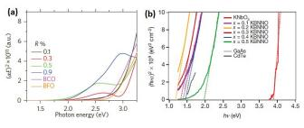
**Fig. 11** ( $\alpha E$ )<sup>2</sup>vs *E* plot of the UV-vis absorption spectra of (a) BFCO (reproduced from ref. 34, copyright 2015, Nature Publishing Group) and (b) KBNNO (reproduced from ref. 151, copyright 2013, Nature Publishing Group).
