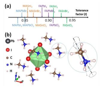
**Fig. 1** (a) Tolerance factors (*t*) of a series of halide perovskites. (b) Crystal structure of MAPbl<sub>3</sub> represented by an ABX<sub>3</sub> primitive unit cell. The right panel of b shows the orientational disorder of MA<sup>+</sup> molecules
