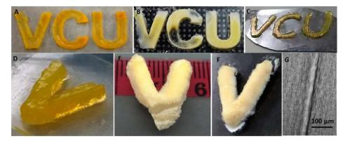
**Figure 2:** Shows letters printed using mask, (a) on laminated paper, (b) on glass, (c) on silicon wafer, (d) on glass, and letter "V" was dried at supercritical conditions and shown as: (e) without substrate, (f) on glass substrate, whereas (g) shows a line printed without mask on glass. The typical thickness of the letters is 2-4 mm whereas each letter has dimensions of 12 mm x 15 mm.
