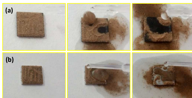
Fig. 11. Self-cleaning property test: soils loaded superhydrophobic surface is cleaned by moving water droplets (a); soils loaded untreated zinc surface is not cleaned by moving water droplets (b).
