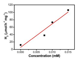
Figure 7. Hydrogen production rates under different concentrations of cobalt-salen
