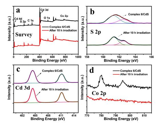
**Figure 4.** (a) XPS survey spectra of the photocatalyst samples. Black plot is for the mixture of CdS NRs and complex **6**. Red plot is the photocatalyst after H<sub>2</sub> production reaction, which was centrifuged and washed by acetonitrile and water after 10 hours of irradiation. (b) High resolution spectra of S 2p. (c) High resolution spectra of Cd 3d. (d) High resolution spectra of Co 2p.
