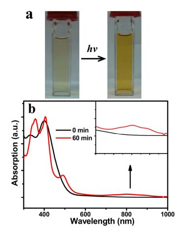
**Figure 6.** (a) Color change and (b) UV-vis absorption spectra of a solution containing  $1.6 \times 10^{-2}$  M TEOA,  $1.1 \times 10^{-5}$  M Pt chromophore, and  $3.0 \times 10^{-4}$  M complex **6** in DMF (5% water) under inert atmosphere. Black plot is from the solution without irradiation and red plot is from the solution after photocatalysis for 60 min. After 1 hour illumination, the color of the solution had turned from light yellow to dark yellow.
