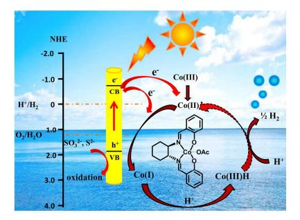
Scheme 3. A possible mechanism for  $H_2$  production in the present reaction system.
