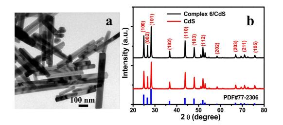
**Figure 1.** (a) TEM image of CdS NRs; (b) Powder XRD pattern of CdS NRs (red plot) and cobalt-salen complex **6** mixed with CdS NRs (1.4 wt % of cobalt in the composite). Blue plot is the standard XRD pattern, CdS-PDF#77-2306.
