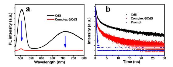
**Figure 5.** (a) Photoluminescence spectra and (b) time-resolved photoluminescence decay spectra of CdS NRs (black plot) and complex **6**/CdS NRs (red plot) excited at a wavelength of 405 nm. The complex **6** and CdS NRs were dissolved in acetonitrile and then dropped using a pipette onto a glass plate to form a film.
