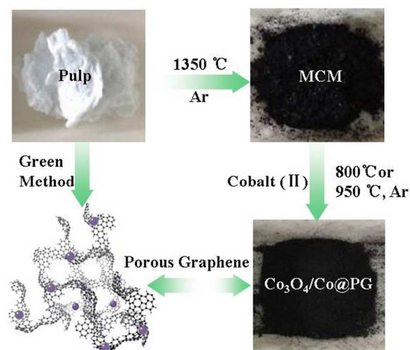
Scheme 1 Schematic procedure for functional porous graphene ( \text{Co}_3\text{O}_4/\text{Co}@PG ) from waste paper (MCM stands for microporous carbonaceous material and PG stands for porous graphene).
