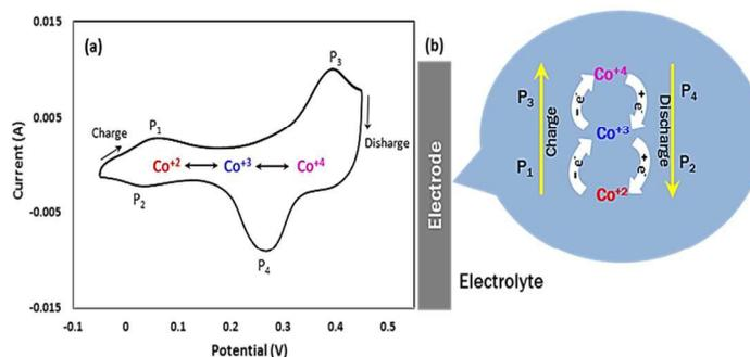
**Fig. 6** (a) Typical CV curve of CC-based electrode taken at a scan rate of  $20 \text{ mV s}^{-1}$  and (b) schematic illustration of redox reactions of cobalt cations on the surface of the electrode in KOH electrolyte.
