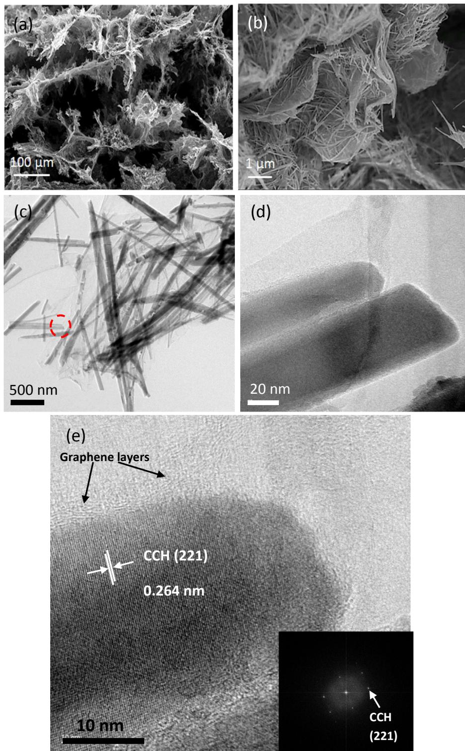
**Fig. 3** (a, b) SEM, (c, d) TEM images and (e) HRTEM and FFT pattern of CCH nanowire single crystals on graphene of CCH/GA-2 composite.
