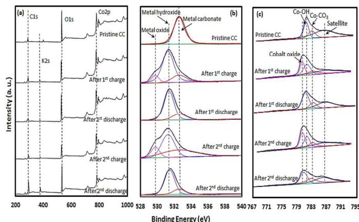
**Fig. 5** XPS spectra of pristine CC electrode after the first and second charge and discharge cycles: (a) general spectra; (b) deconvoluted O 1s spectra and (c) deconvoluted Co 2p spectra.
