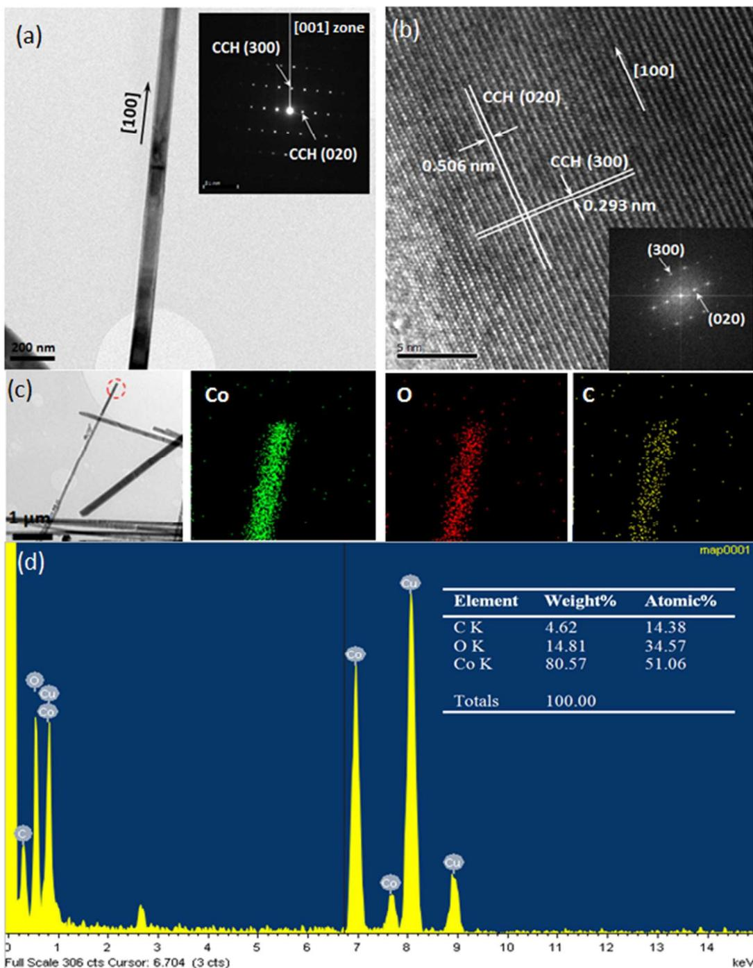
**Fig. 2** TEM images of CCH/GA-0 (without graphene): (a) CCH nanowires and SAED pattern in the inset; (b) HRTEM of a CCH single crystal and FFT pattern in the inset; (c) elemental mapping; and (d) EDS analysis.
