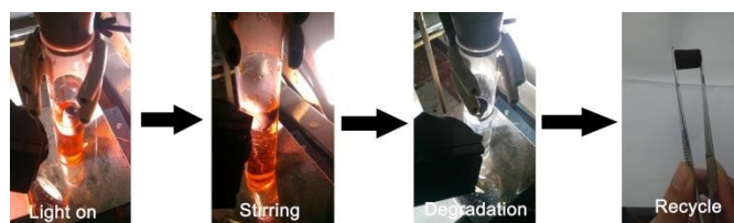
Fig. 7 Photographs of the cycle test of \text{Fe}_2\text{O}_3/\text{GAs} for the solar-driven Photo-Fenton reaction.
