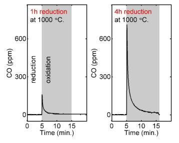
Figure 7. Carbon monoxide production measured by NDIR detector for  $La_{0.6}Sr_{0.4}Cr_{0.8}Co_{0.2}O_{3-\delta}$  by splitting  $CO_2$  in a fluidized bed reactor in a temperature cycle of 800 to  $1000^{\circ}C$ . The material was reduced at  $1000^{\circ}C$  for 1 h and 4 h in the first and second cycle respectively before it was re-oxidized by  $CO_2$  at  $800^{\circ}C$ . CO production yields are 10 and  $63\mu$ mol/g for the short and longer reduction cycle respectively.
