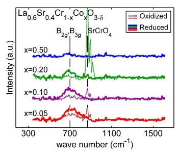
Figure 4. Raman Spectra of  $La_{0.6}Sr_{0.4}Cr_{1-x}Co_xO_{3-\delta}$  with x=0.05, 0.10, 0.20, and 0.50 for as-synthesized (oxidized) and thermochemically cycled powders (reduced). Broad peak at ~700cm<sup>-1</sup> is assigned to  $B_{2g}$  and  $B_{3g}$  breathing modes. The feature at 870cm<sup>-1</sup> visible only for some spots in the oxidized samples are assigned to impurity phase  $SrCrO_4$ .
