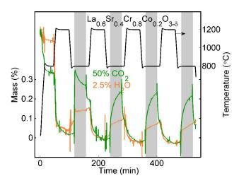
Figure 8. Thermogravimetric cycling data of  $La_{0.6}Sr_{0.4}Cr_{0.8}Co_{0.2}O_{3-\delta}$  for two experiments with reduction in argon and re-oxidation with either 50%  $CO_2$  or 2.5%  $H_2O$  in argon. Outliers are artefacts arising as a consequence of the high sensitivity of the thermogravimetric analyser. Reproducible cycles are observed for cycle 2-4 for re-oxidation with both water and carbon dioxide.
