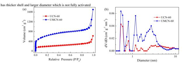
Fig. 3 Nitrogen absorption-desorption isotherms (a) and pore size distributions curve (b) of UCN-60 and UMCN-60.
