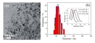
Fig. 1 A typical TEM image (a) and DLS data (b) of P/T-60 polymer colloids (The inset shows fitted curves of DLS data of P/T-30, P/T-60 and P/T-120).
