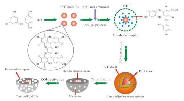
Fig.4 Schematic synthesis of 3D core-shell UMCNs with regular ultramicropores in the cores and abundant micropores in the shells.
