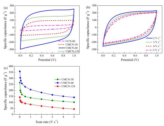
Fig. 7 CV curves of UCN and UMCN electrodes at a scan rate of 1000 mV s<sup>-1</sup> (a), CV curves of the UCN-60 electrode at various scan s rates (b), and the relationship between the specific capacitances of UMCN electrodes and the scan rates (c).
