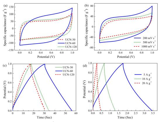
Fig. 5 CV curves of UCN electrodes at 100 mV s<sup>-1</sup> (a), CV curves of UCN-60 electrode at various scan rates (b), GCD curves of UCN 5 electrodes at 1.0 A g<sup>-1</sup> (c) and GCD curves of UCN-60 electrode CV at different current densities (d) in 6 M KOH electrolyte solution.
