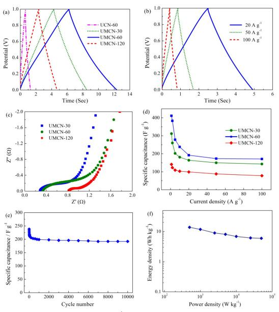
5 Fig. 8 GCD curves of UCN and UMCN electrodes at 10 A g<sup>-1</sup> (a), GCD curves of UCN-60 electrode CV at various current densities (b), Nyquist plots of UCN electrodes (c), the relationship between the specific capacitances of UMCN electrodes and the scan rates (d), Long-term cycle stability of UMCN-60 electrode at 10 A g<sup>-1</sup> (e), and Ragone plots of the UMCN-60 based asymmetric capacitor (f).
